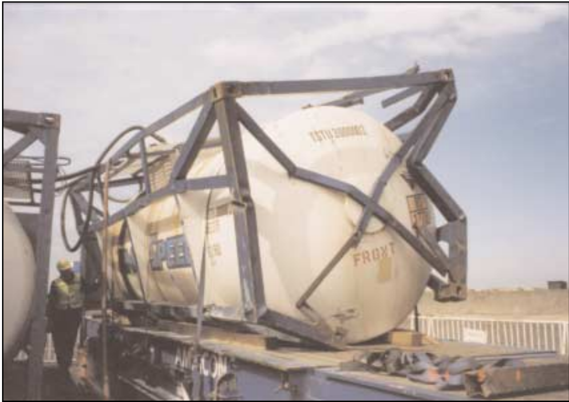
Damaged front end frame
