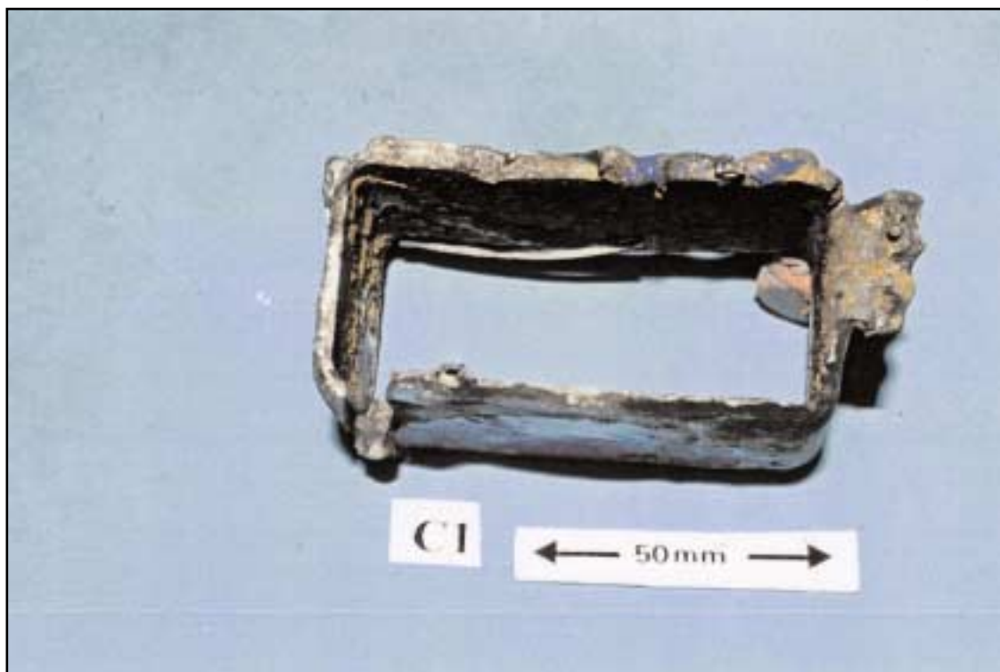
Failed weld repair on front diagonal
