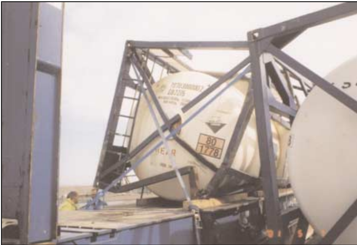
Damaged rear end frame
