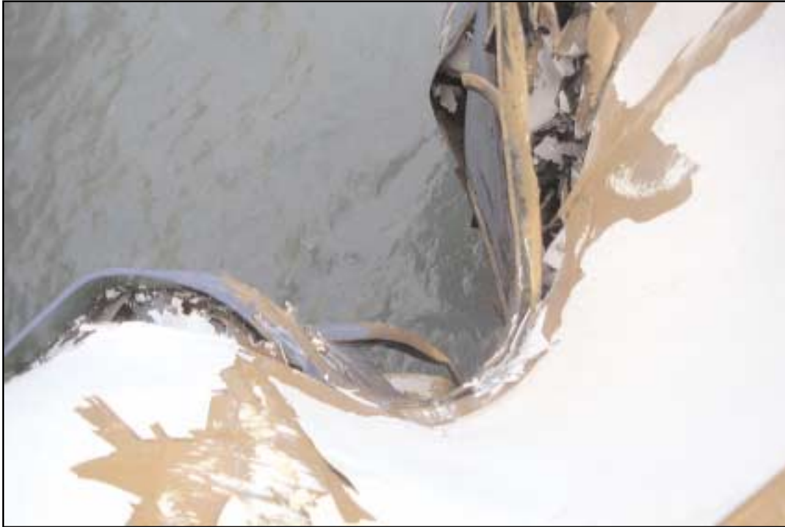
Hampoel damage (looking down from poop) (Note shape of Atlantic Mermaid's bow embedded in stern of Hampoel )
