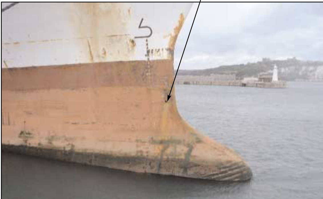
Atlantic Mermaid damage
