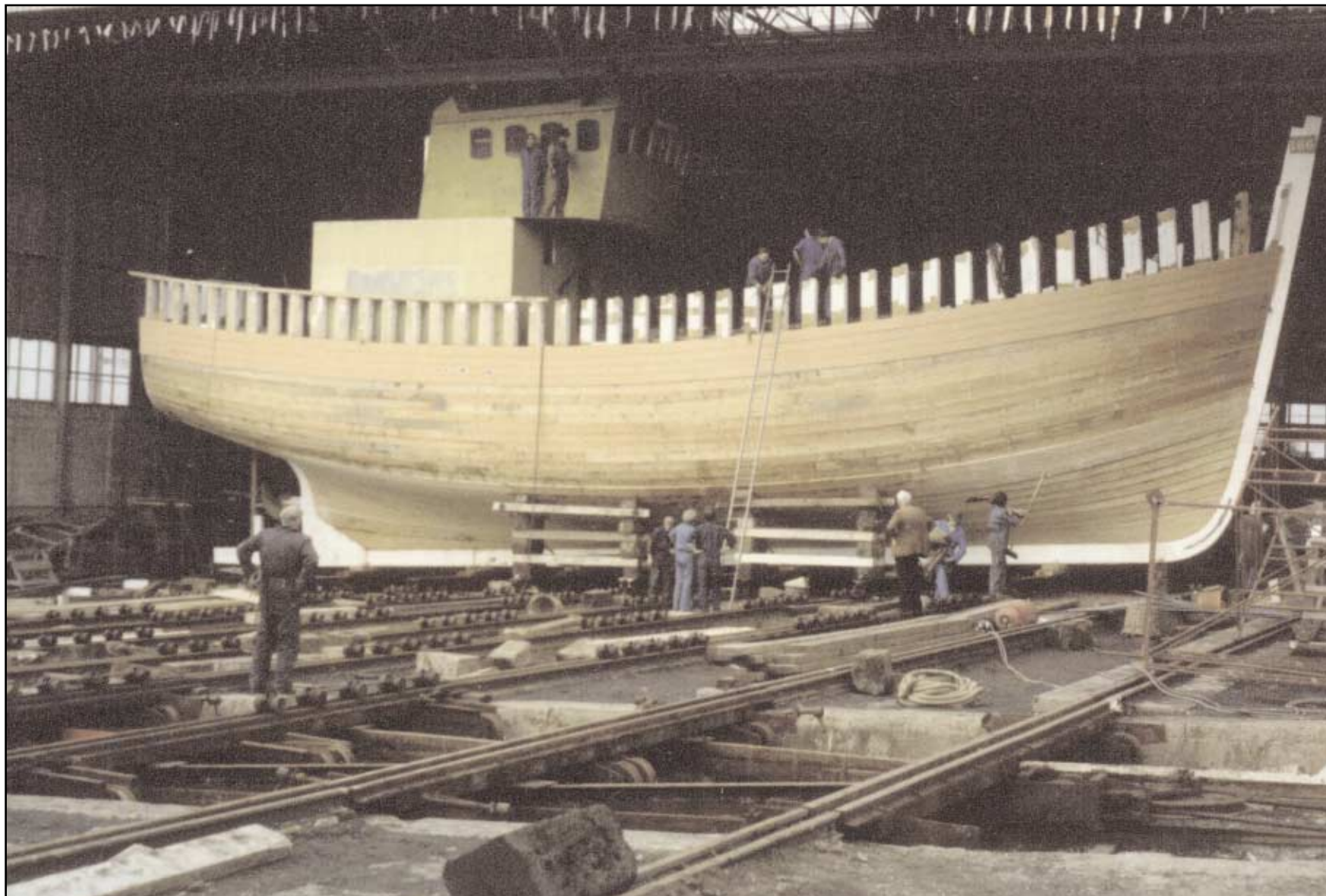
Constant Faith showing wooden construction
