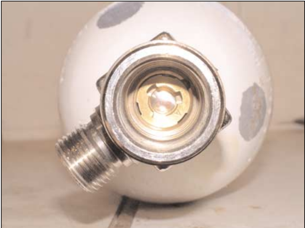
An end view of a gas cylinder with the diaphragm in place
