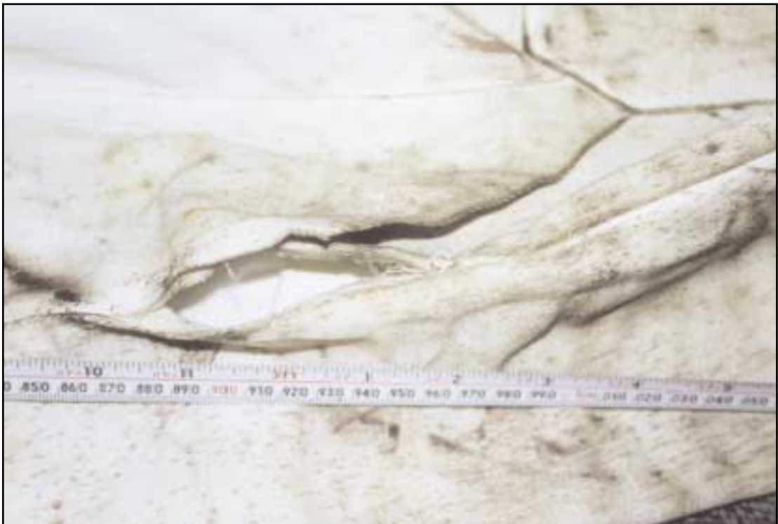
The open seam below the pocket opening
