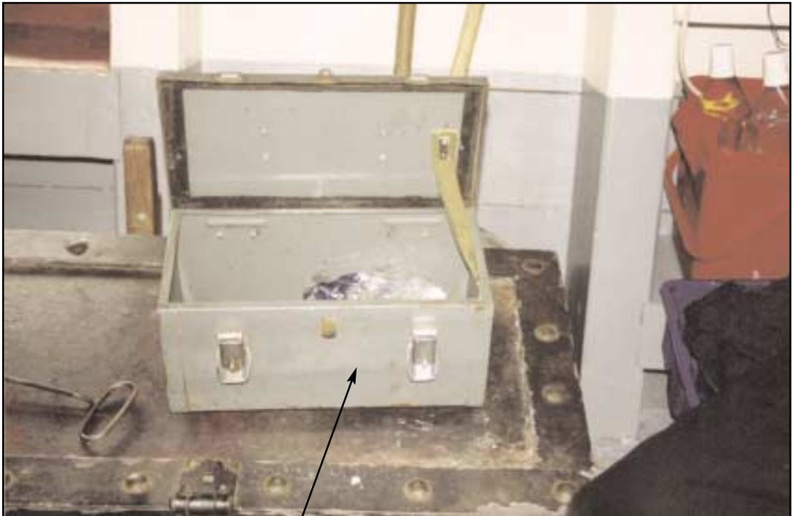
Fireproof box for transporting charges on to deck
