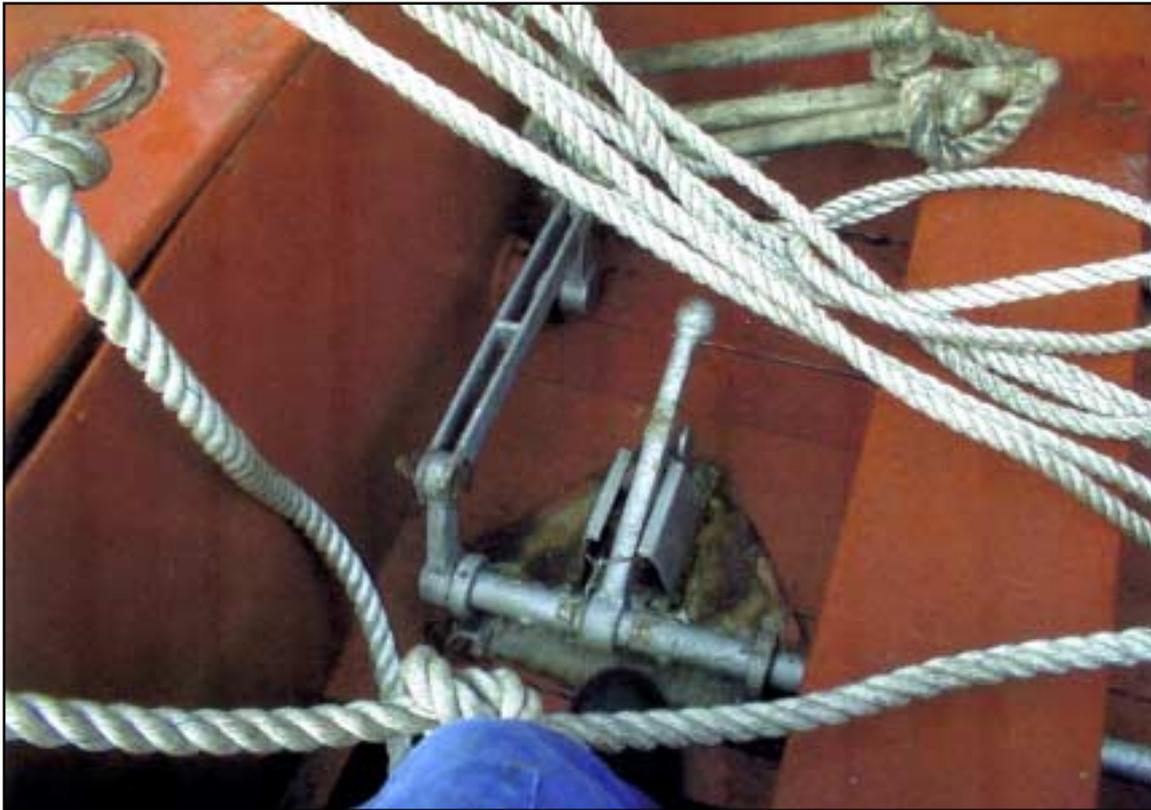
Releasing lever with safety pin missing
