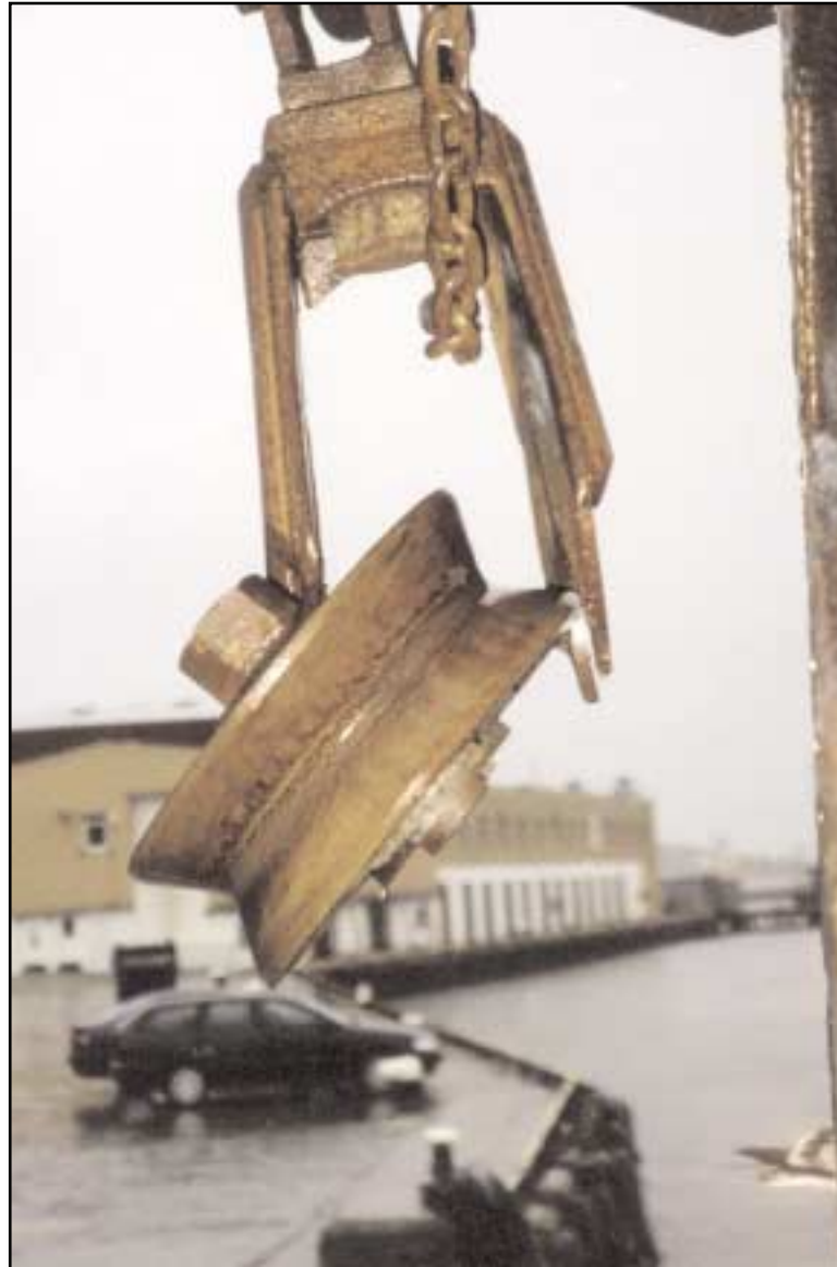
The starboard main warp hanging block in-situ onboard Ocean Star
