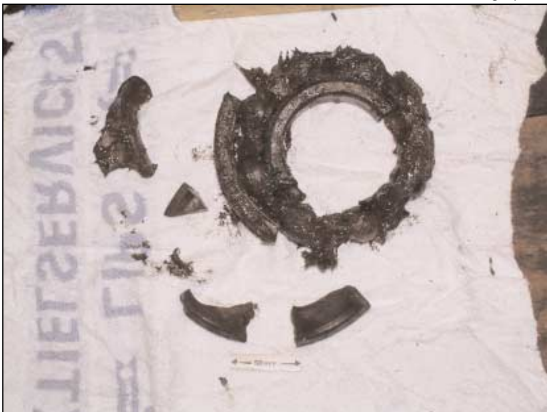
The inboard inner and outer ball races removed from the roller
