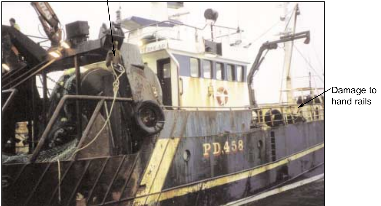
A view of Ocean Star and of the broken starboard main warp block
