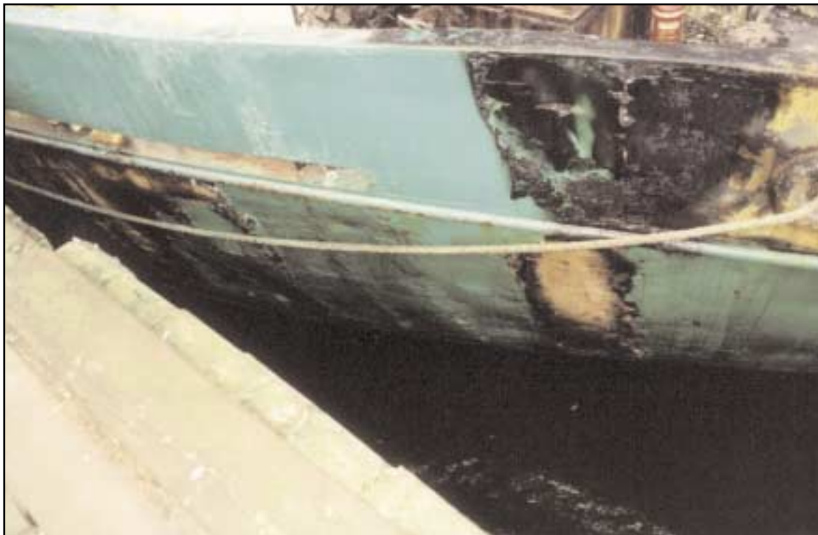
Port quarter showing "hot spot" on hull
