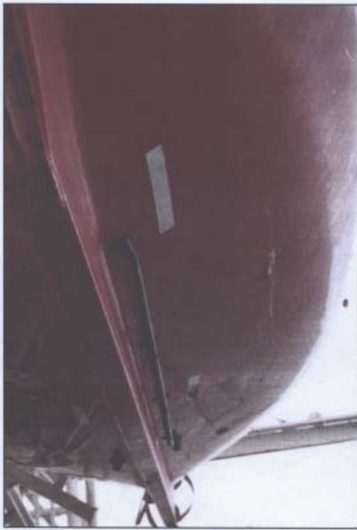
Figure 14 - Damage to hull due to striking deck equipment during fall
