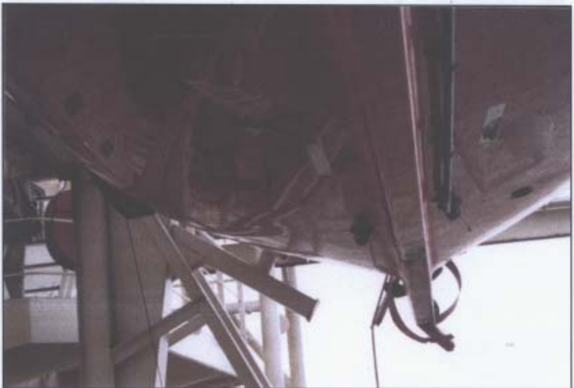
Figure 14 - Damage to hull due to striking deck equipment during fall
