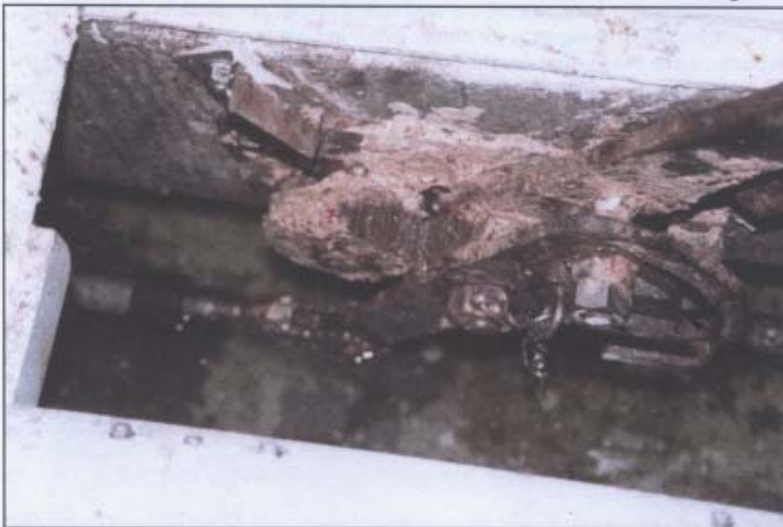
Close-up view of release gear showing quadrant in reset position but locking pin in released position
