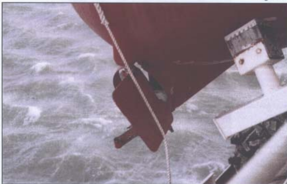
Damage to rudder assembly
