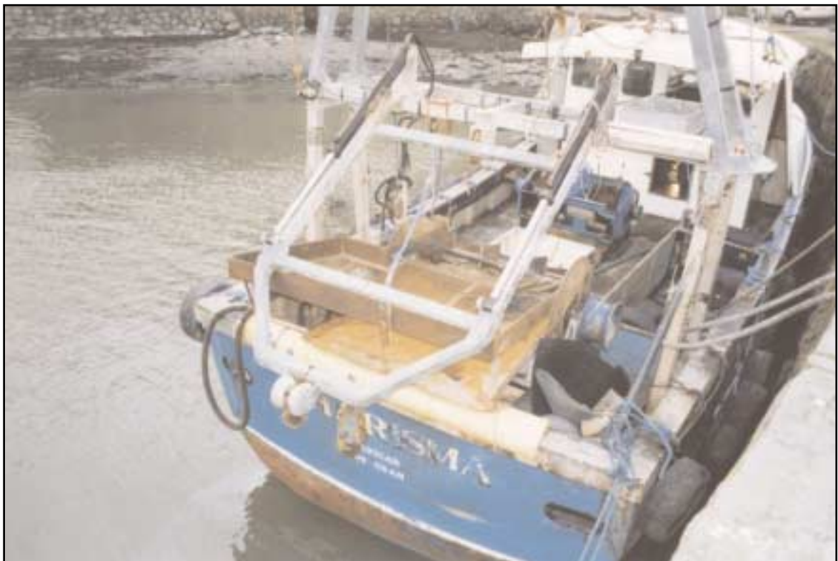
Charisma's stern showing mussel bench and hydraulic gear
