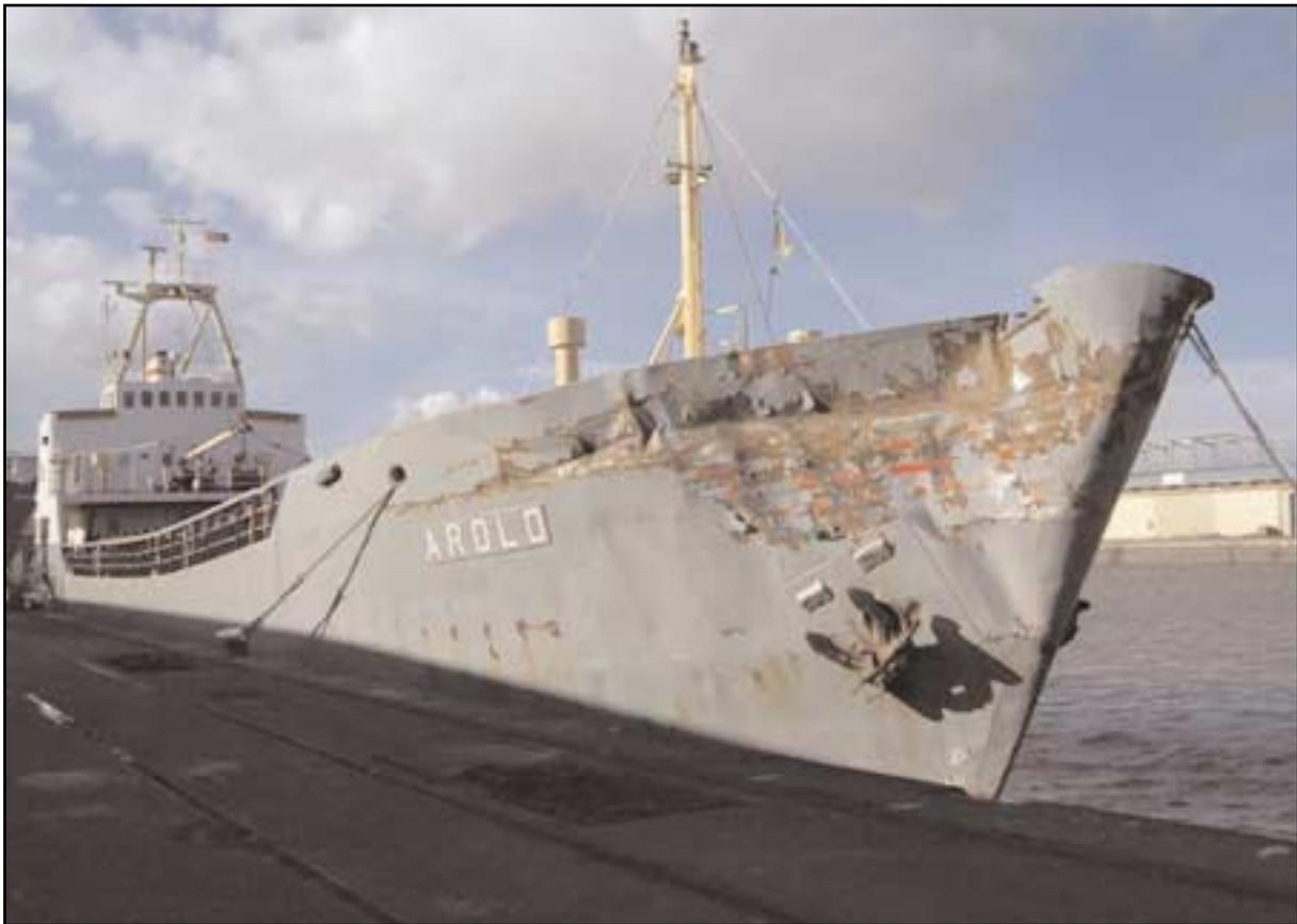
*Arold* berthed at King George Dock, Hull, showing damage to starboard bow
