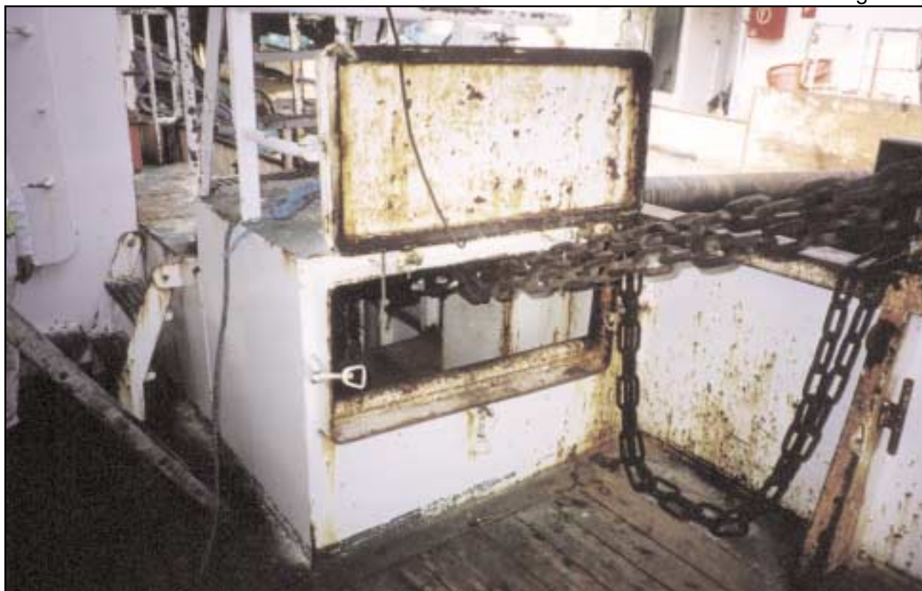
Warp hatch to port winch (downflooding point)
