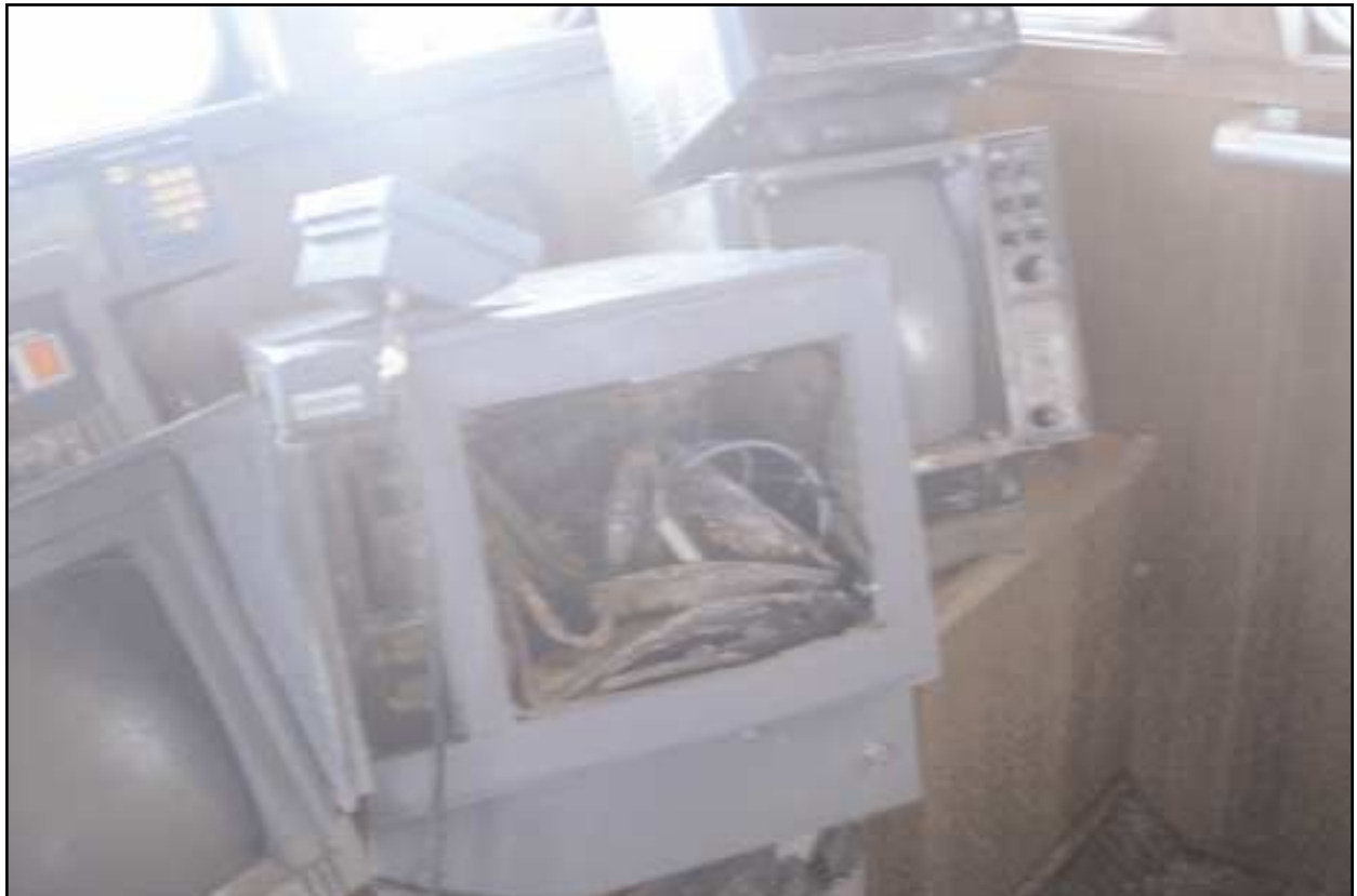
Decca fishplotter with cathode ray tube imploded
