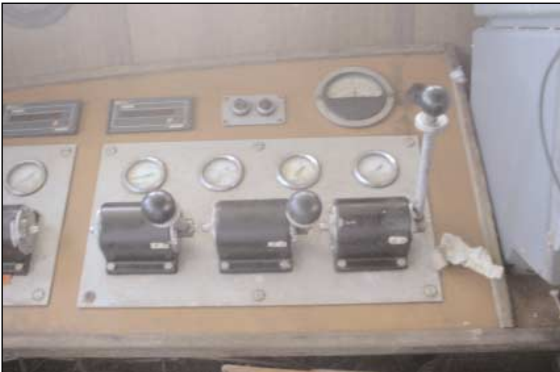
The starboard fishing controls (as found after raising)
