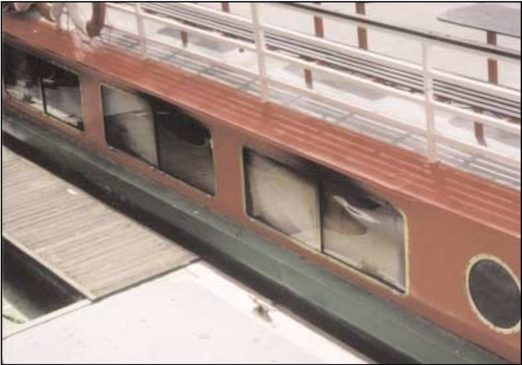
Smoke and heat damage to the side windows in the saloon
