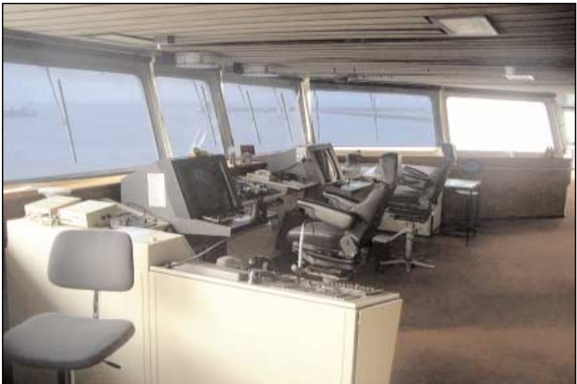
The central manoeuvring console
