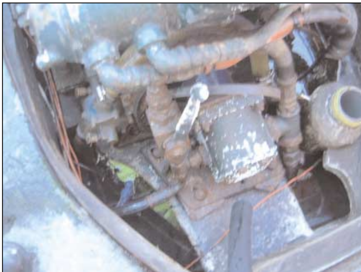
Photograph showing the position of the hydraulic control lever
