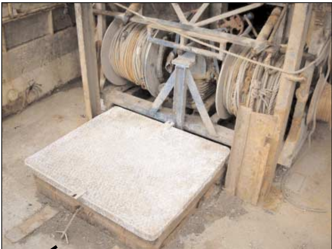
Amber main winch and fish hatch
