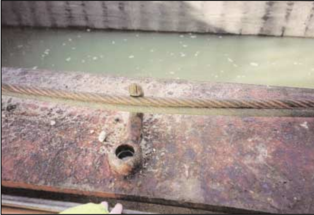
View of port outhaul wire hung off retaining hook
