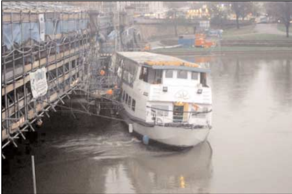
Vessel fast to bridge on Saturday 16th, pm (note flow by bow)
