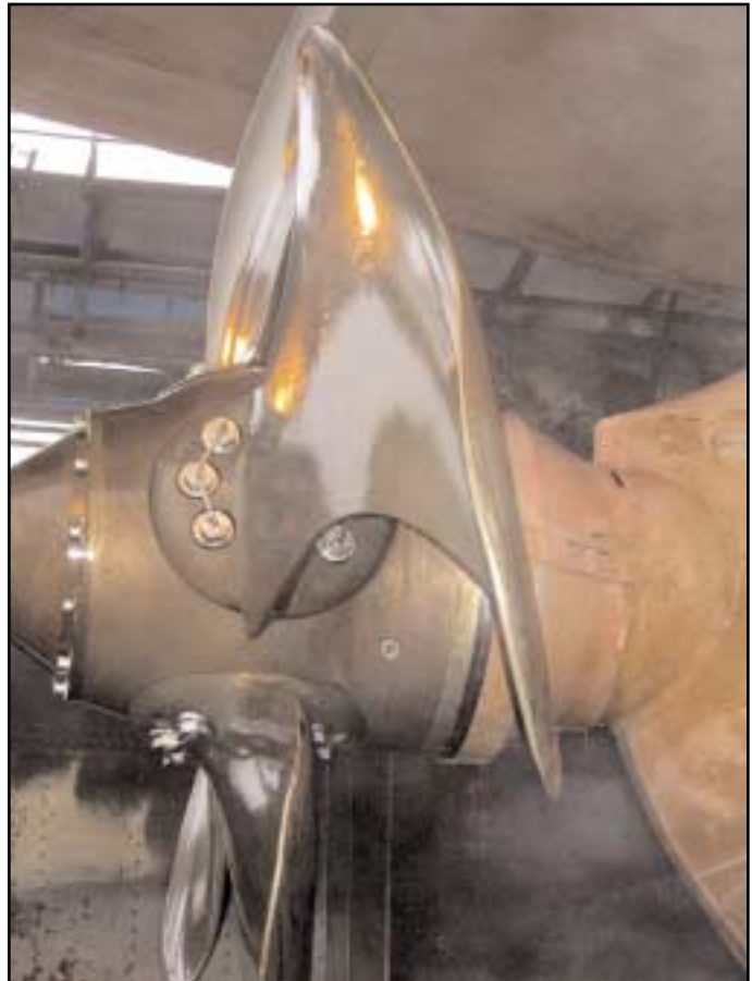
Photograph of the damage to the propeller blades
