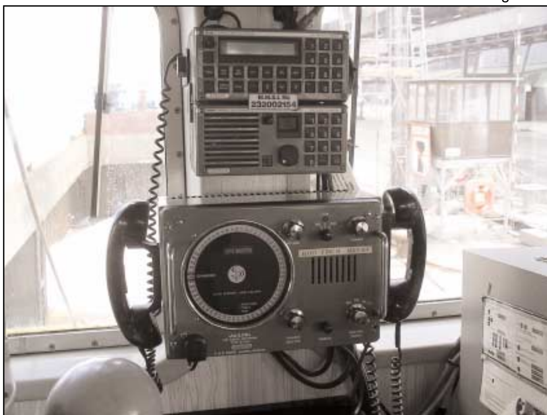
Photograph of the two VHF radios on the bridge of Hoo Finch
