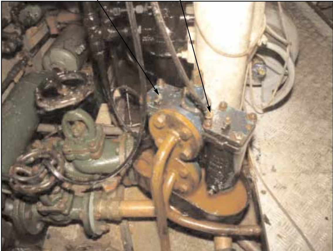
Main engine duplex fuel oil filter arrangement
