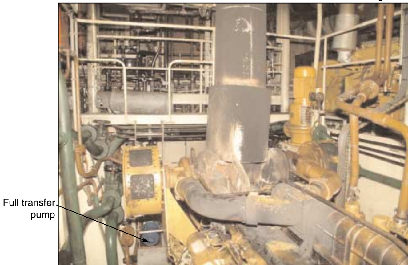
Position of fuel oil transfer pump in relation to main engine
