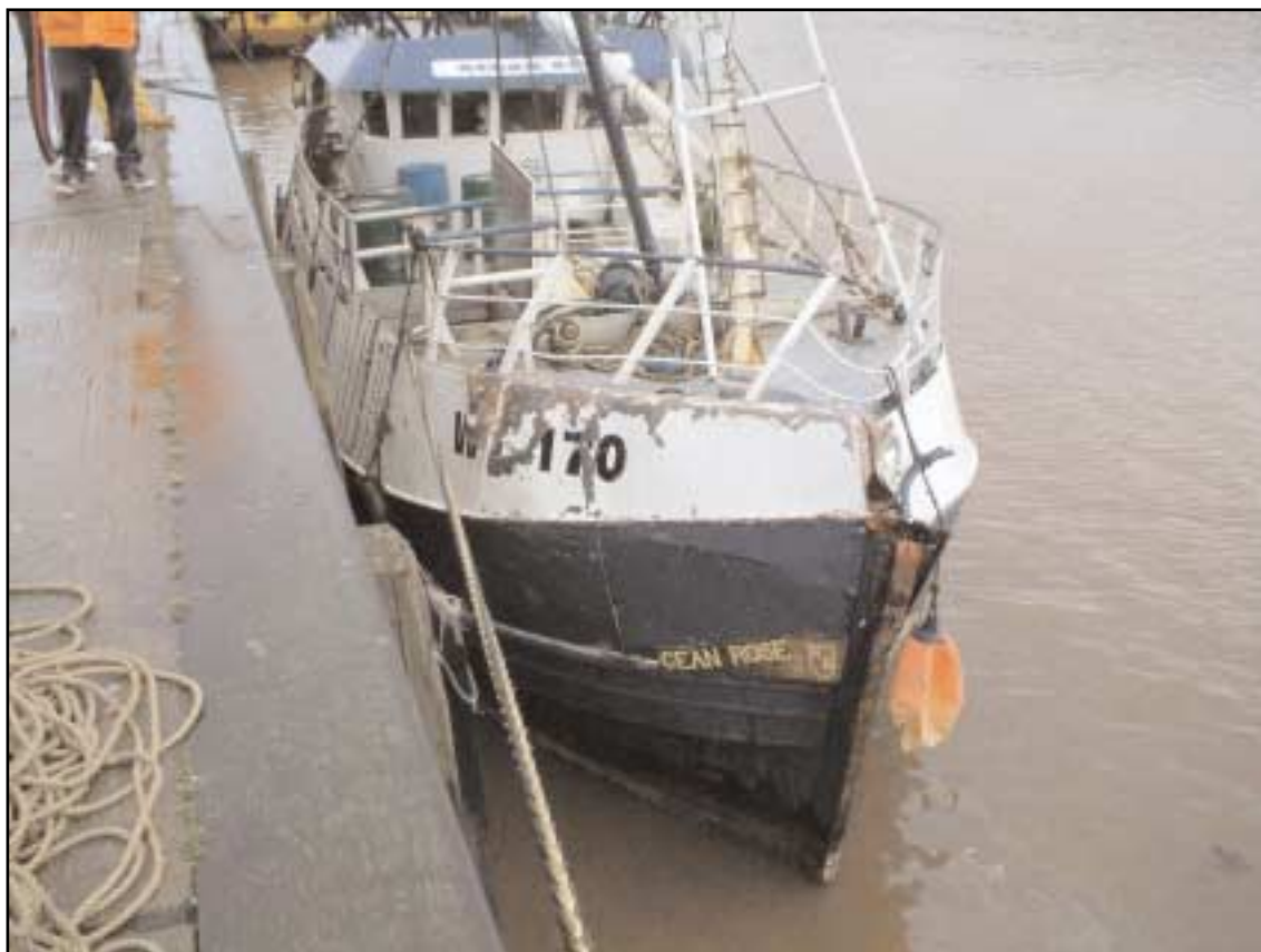
Damage to Ocean Rose - forward
