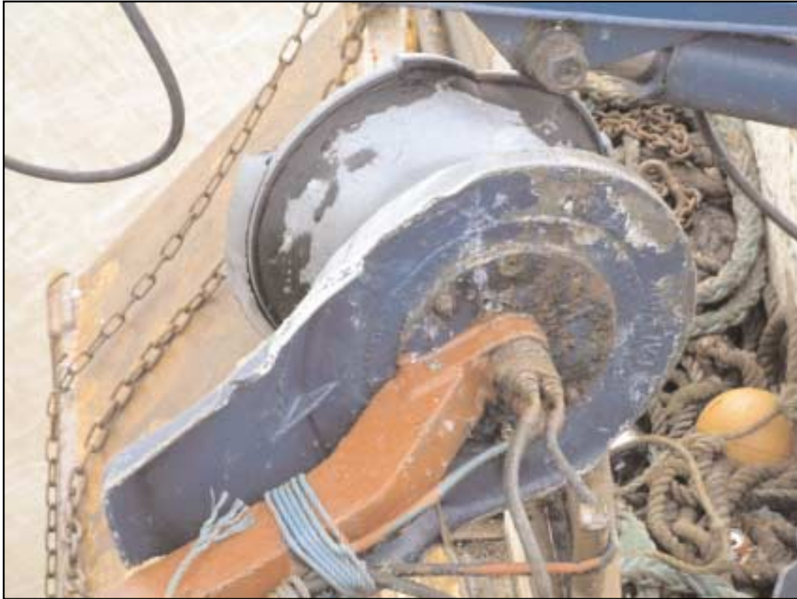
Photograph showing damage to power block
