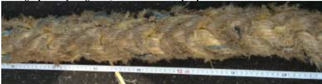
Photograph 5 Eye segment, 12 metres from eye splice
