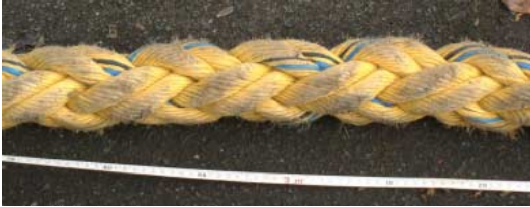
Photograph 3 Eye segment, 3 metres from eye splice
