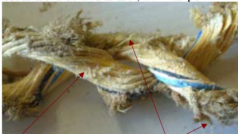
Photograph 16 Internal SOS abrasion and external abrasion, 'within' sample
