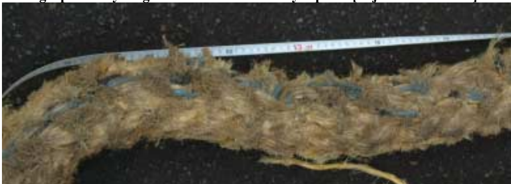
Photograph 6 Eye segment 13 metres from eye splice [adjacent to failure]
