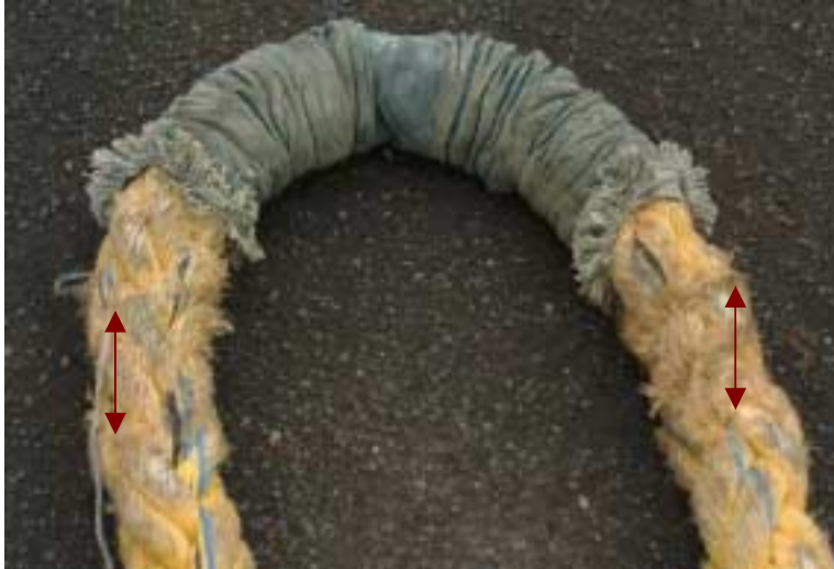
Photograph 9 Eye showing positions of excessive abrasion
