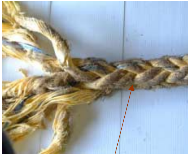
Photograph 10 View of upper face of rope close to fail zone, non-eye segment, showing severe abrasion
