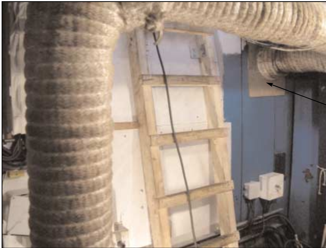
Main engine exhaust passing through engine room/accommodation area bulkhead
