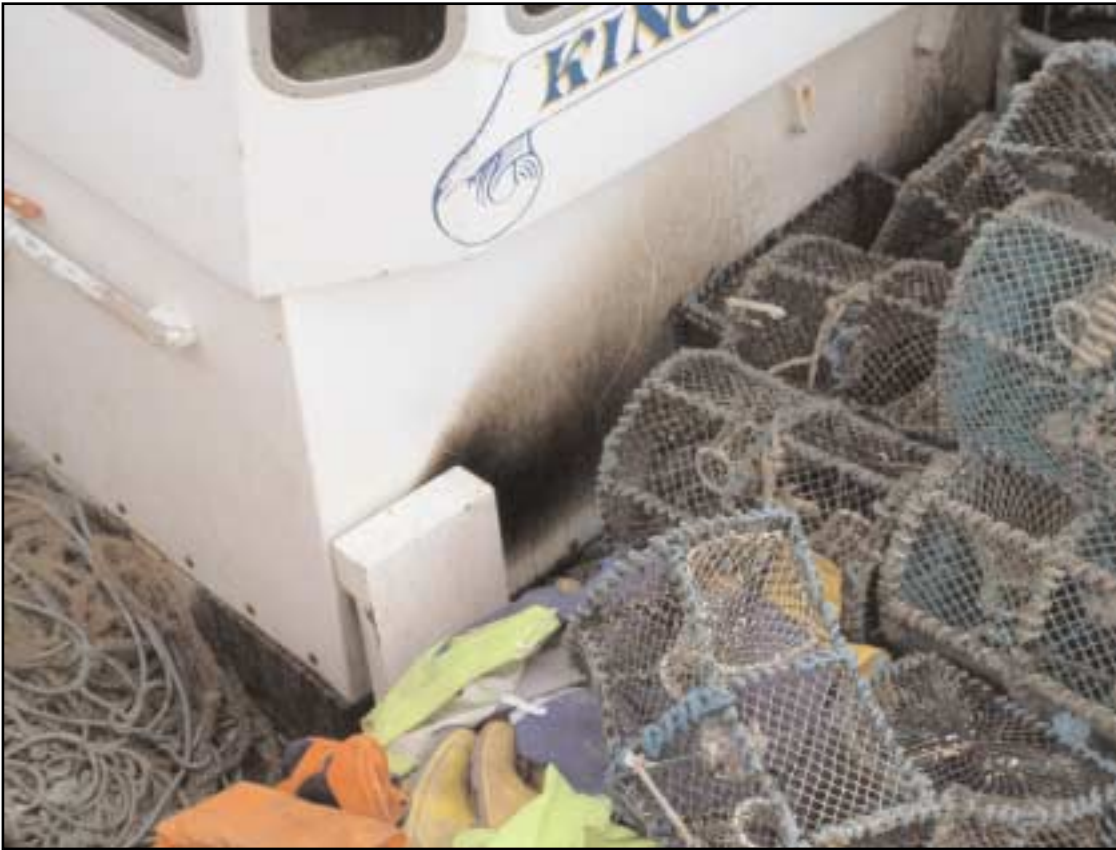
Creel obstruction of engine room vents
