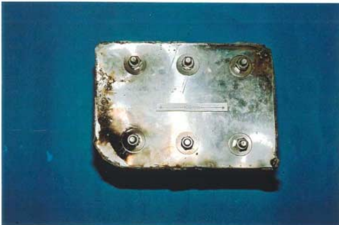
Figure 6: Underside of detached insert plate, showing nut and locking nut securing arrangement.
