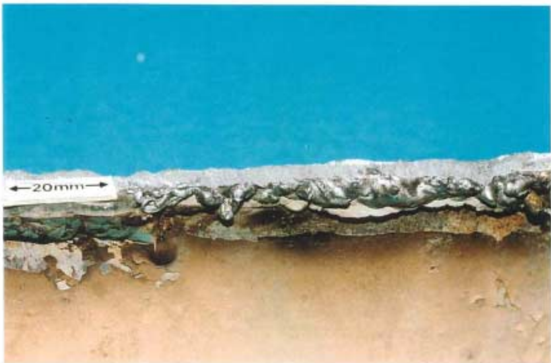
Figure 24: Detail of above, showing area of excessive root penetration.
