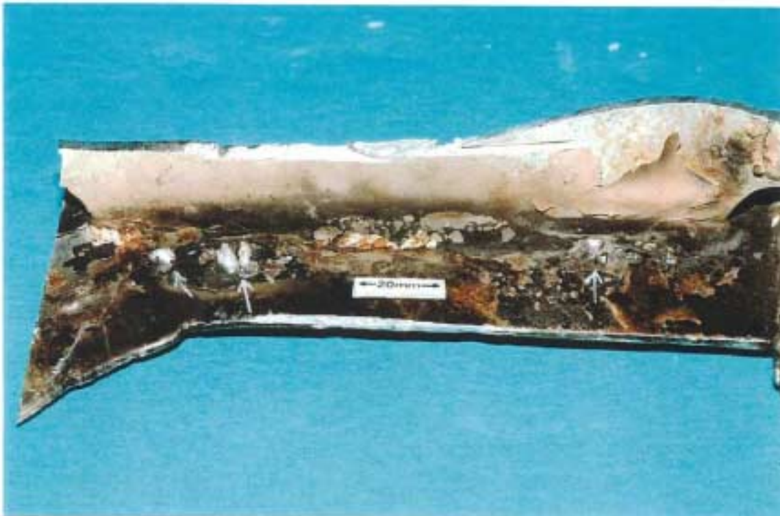
Figure 22: Under-floor forward section, showing local excess penetration or burn-through the chequer plate (arrowed) from the insert weld to the upper chequer plate surface.
