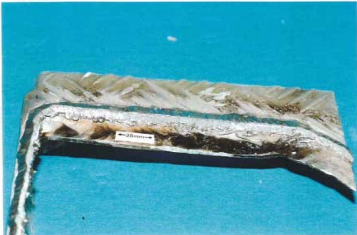
Figure 20: Under-side fractured forward weld section.
