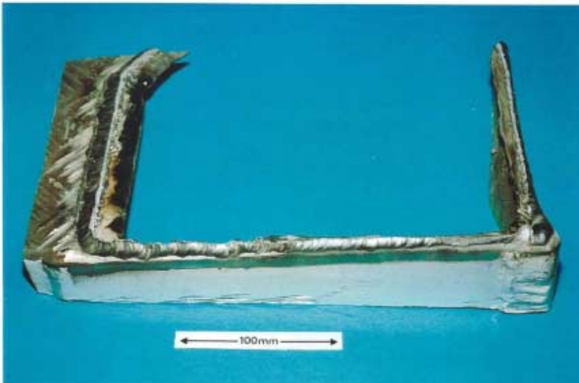
Figure 18: Underside fracture half comprising the forward end, outboard side and aft ends only.
