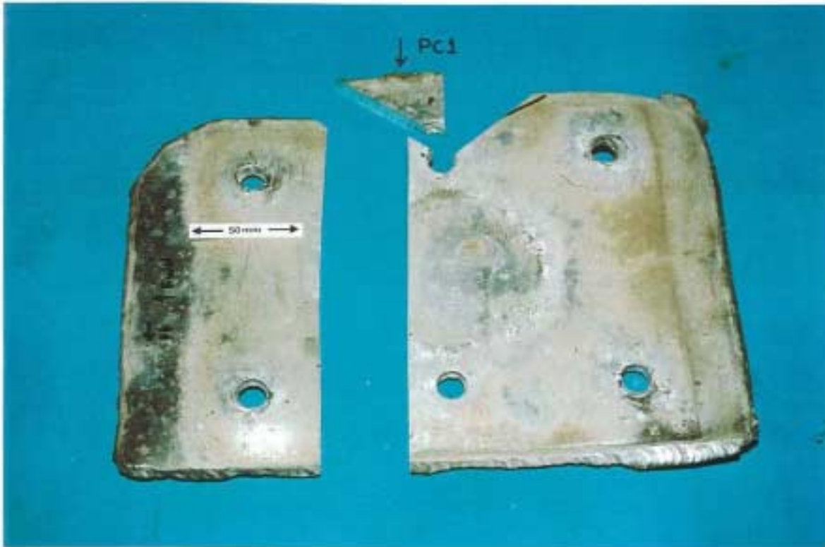
Figure 27: Sample (PC1) removed from inboard weld side and which was subjected to detailed examination.
