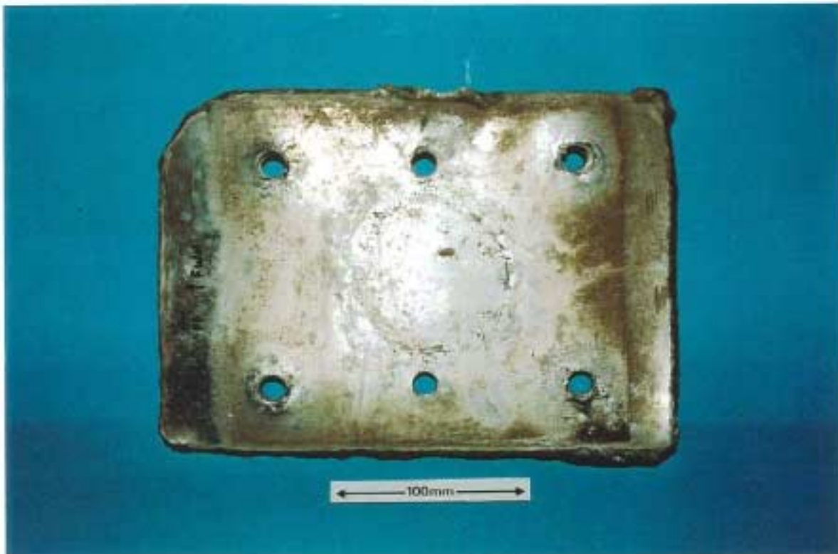
Figure 13: Insert plate, showing bollard base downwards indenting of the aft outboard corner (lower right corner of field).
