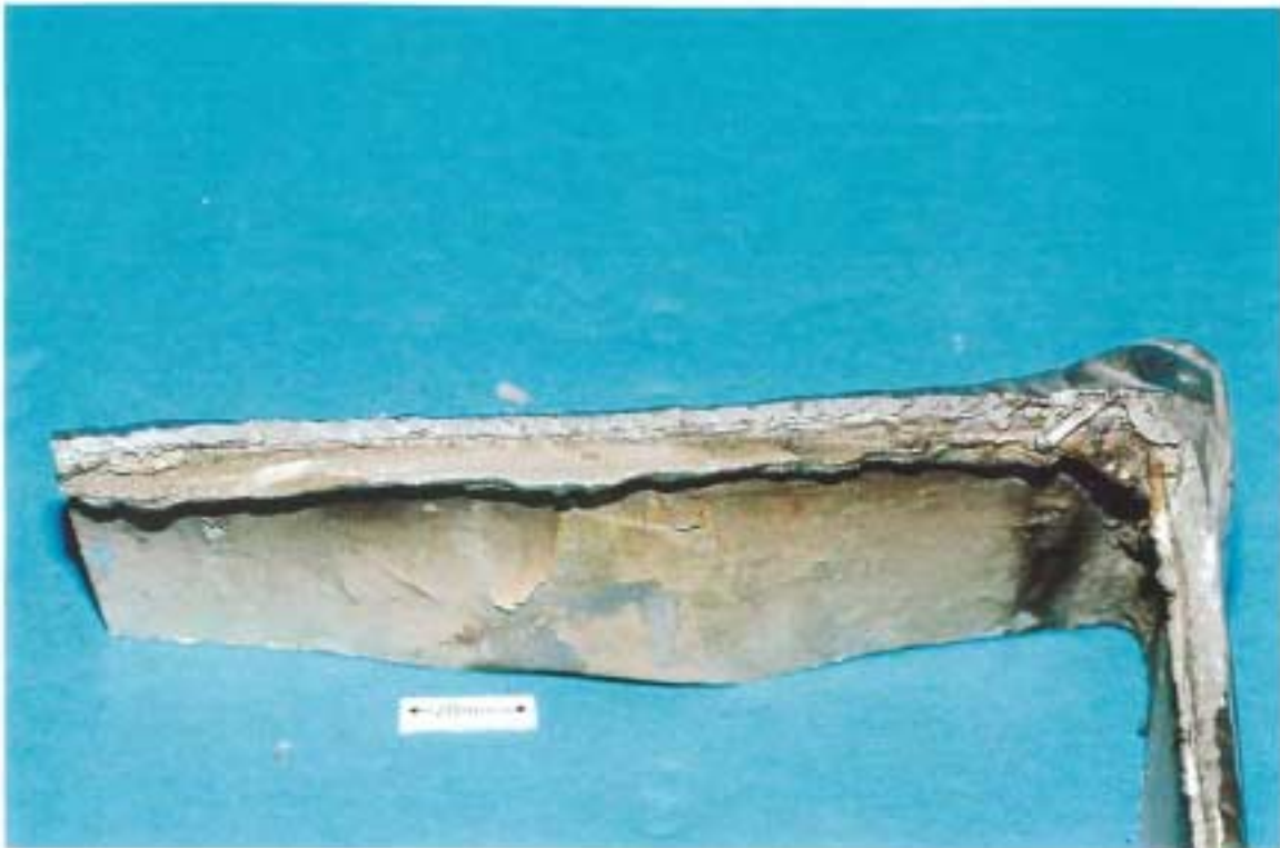
Figure 25: Under-side of fractured aft weld section.
