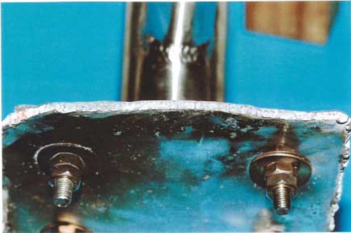
Figure 15: Detail of figure 14, showing fractured weld metal.
