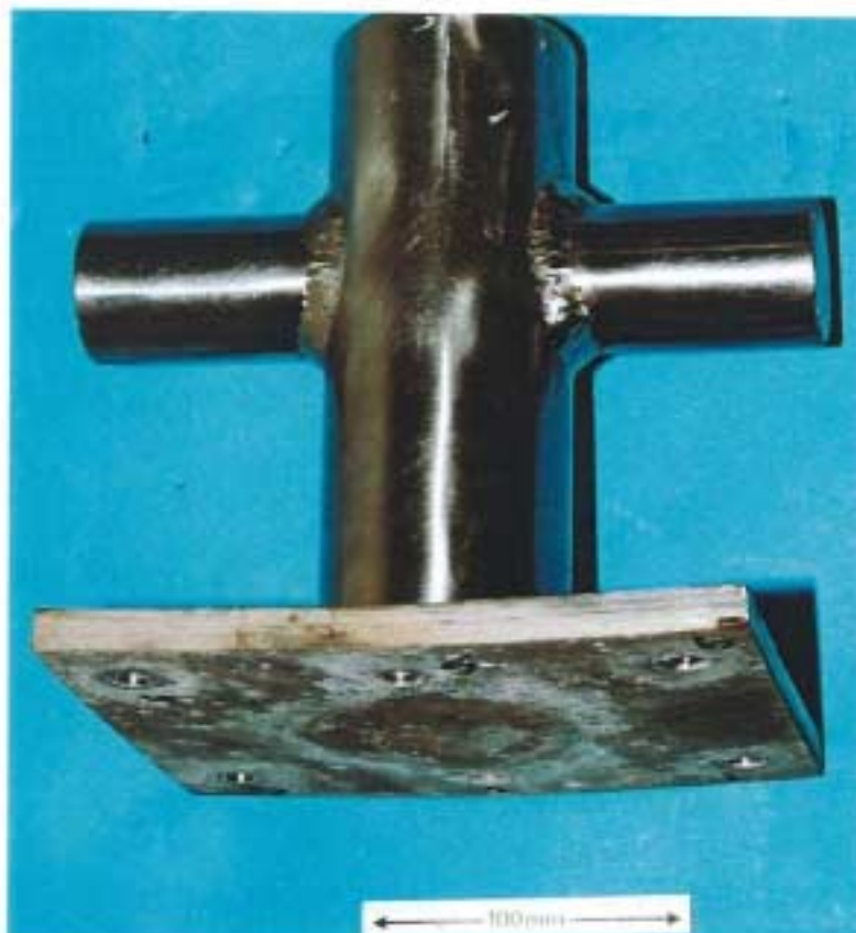
Figure 8: Side view of bollard, showing welding related base plate distortion.
