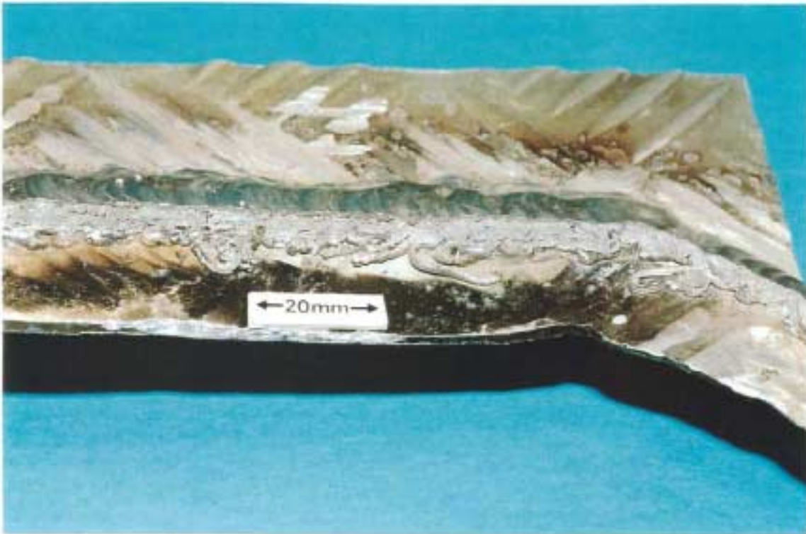
Figure 21: Detail of figure 20, showing unfused root bead roll-through and possible entrapped consumable welding wire in weld root.
