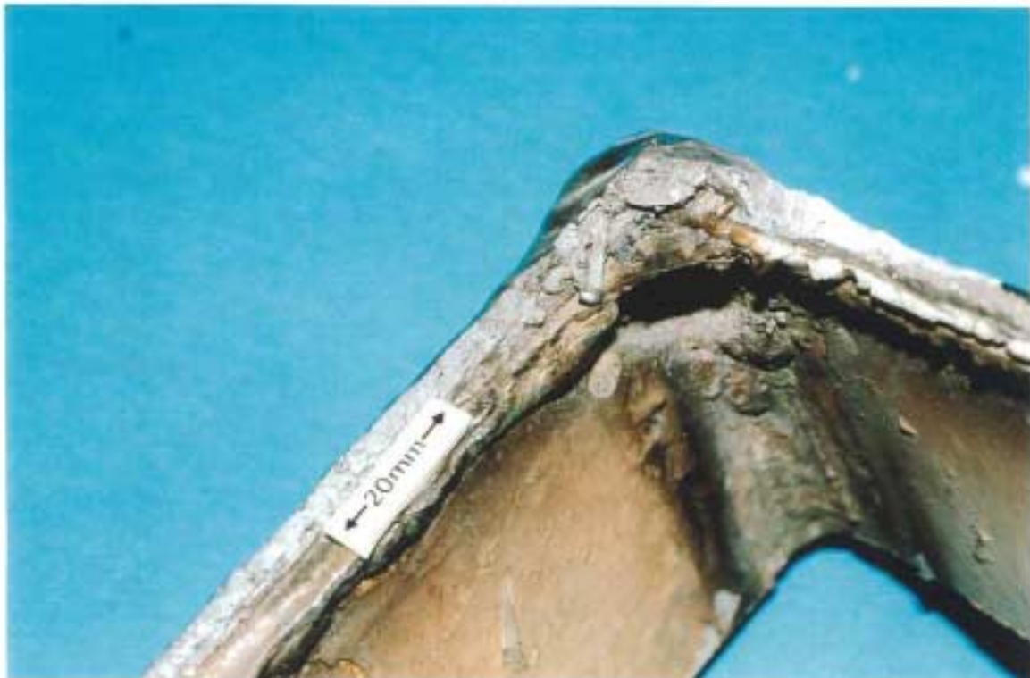
Figure 26: Detail of above, showing weld root defects in the corner transition region from the outboard weld side.
