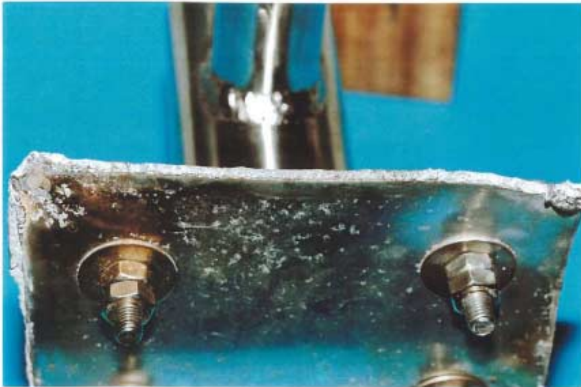
Figure 17: Detail of figure 16, showing fractured weld metal.
