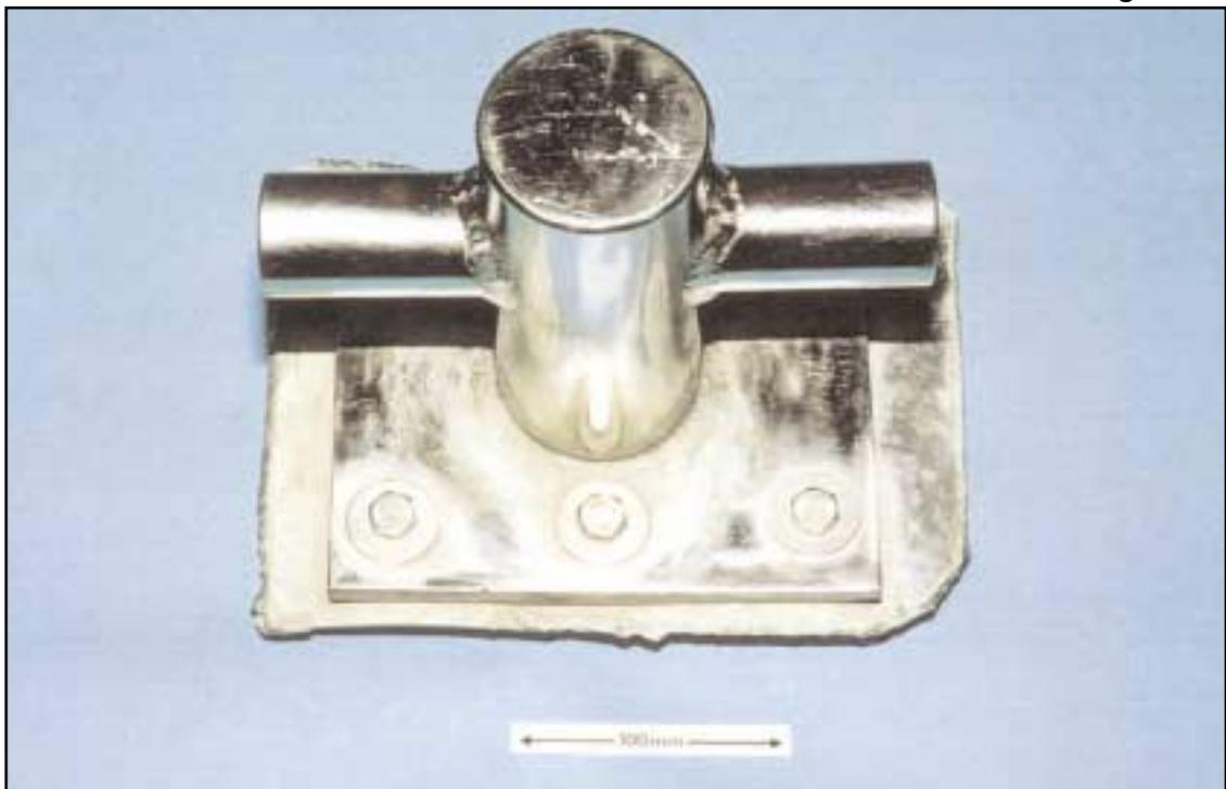
Bollard and insert plate fastening arrangements viewed from inboard side
