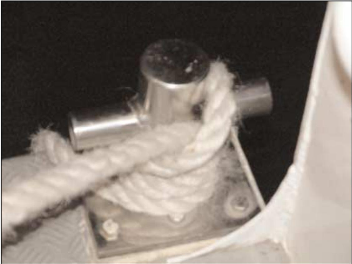
Mooring rope 'pin hitch' arrangement
