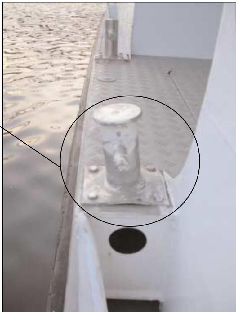
View of Mk1 hollow aluminium bollard
