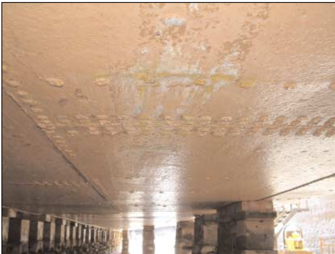
Scrape damage starboard side, looking forward
