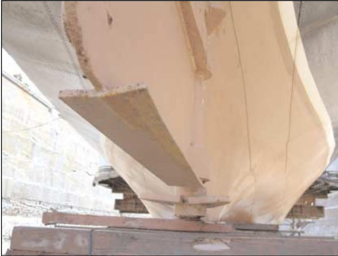
Damage to underside of Waverley's rudder
