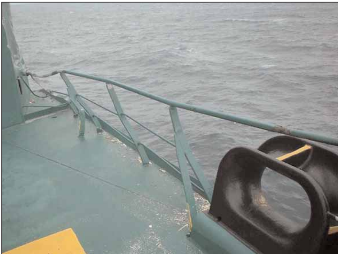
Damaged guardrails - Hyundai Dominion
