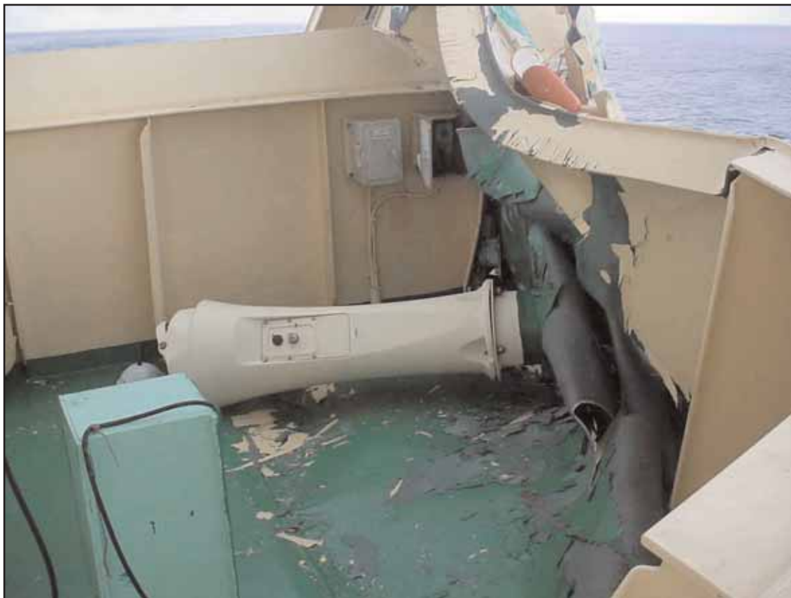
Damaged starboard bridge wing - Sky Hope
