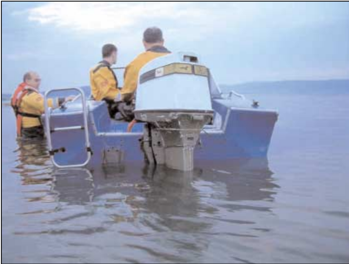
Loading trials - loading condition similar to that just prior to the accident Note: other crew not visible from photograph angle
