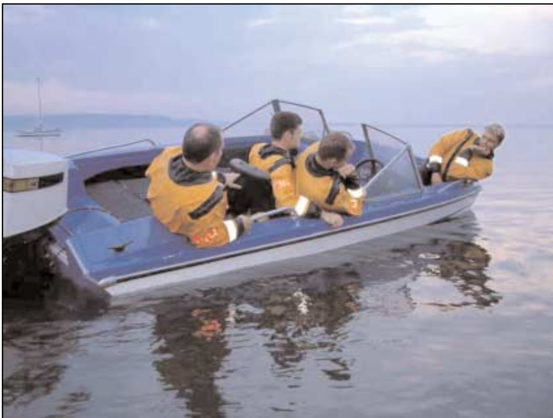
Loading trials - lifeboatmen moved to the starboard side of the boat to assess stability
