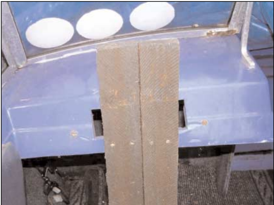
Wood bracket fitted to stow the auxiliary outboard
