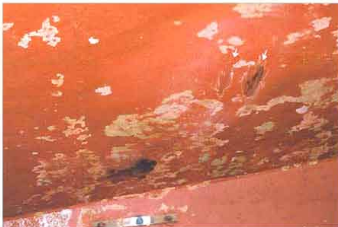
Figure 41: General view of the aft port side crack site (cracks arrowed)
