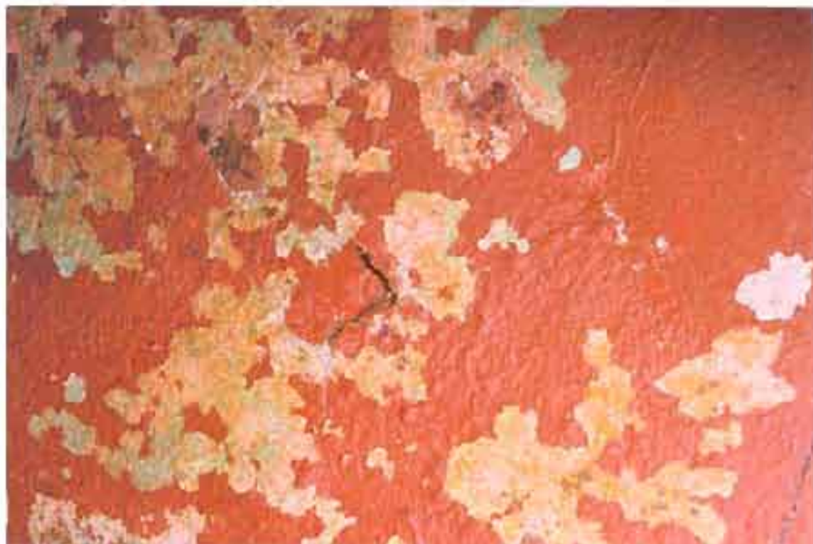
Figure 40: Detail showing extent of port side vee shaped crack mouth gape.
