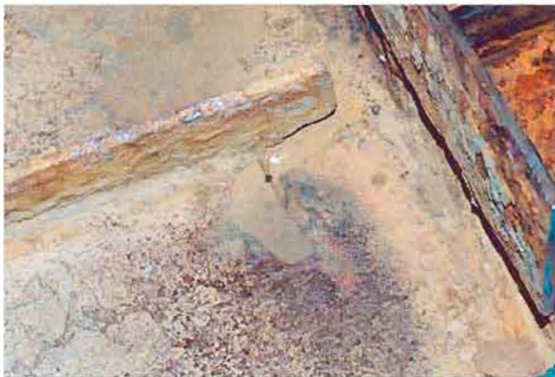
Figure 43: Detail showing crack (arrowed) originating from the fillet weld end
