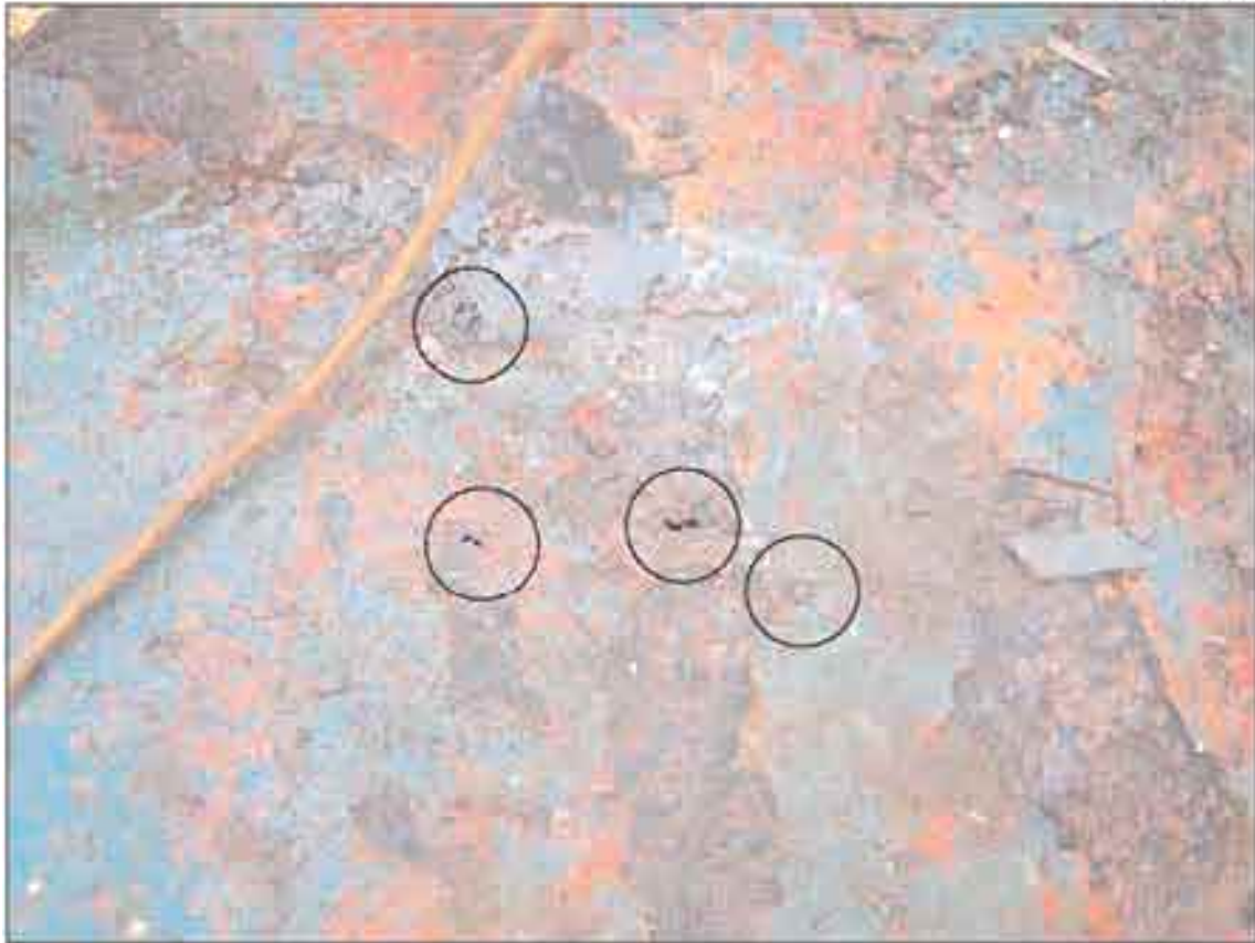
Perforations to upper deck above steering compartment
