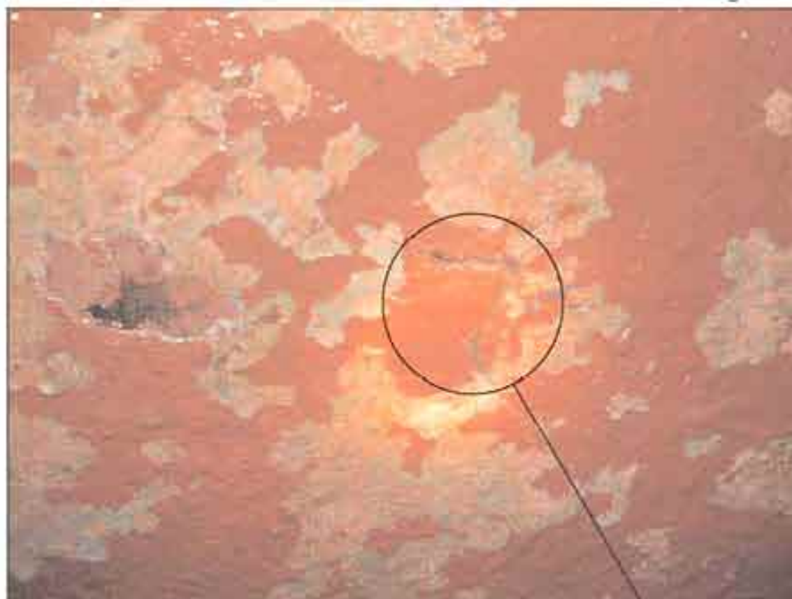
"Vee" split in port side of hull
