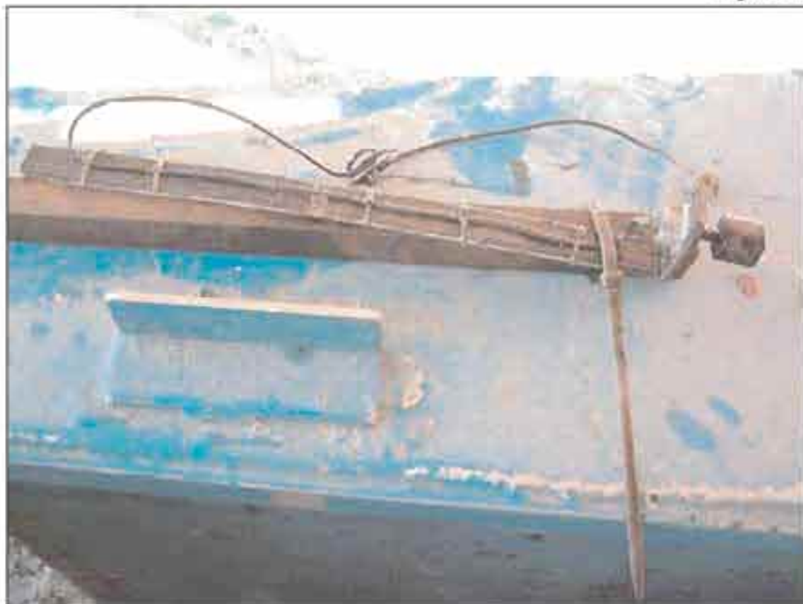
Engine room high level bilge alarm arrangement
