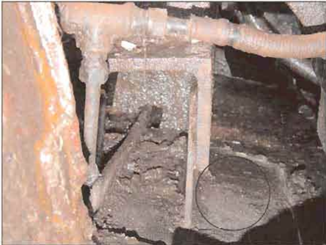
Area of deep pitting in engine room bilge shell plating
