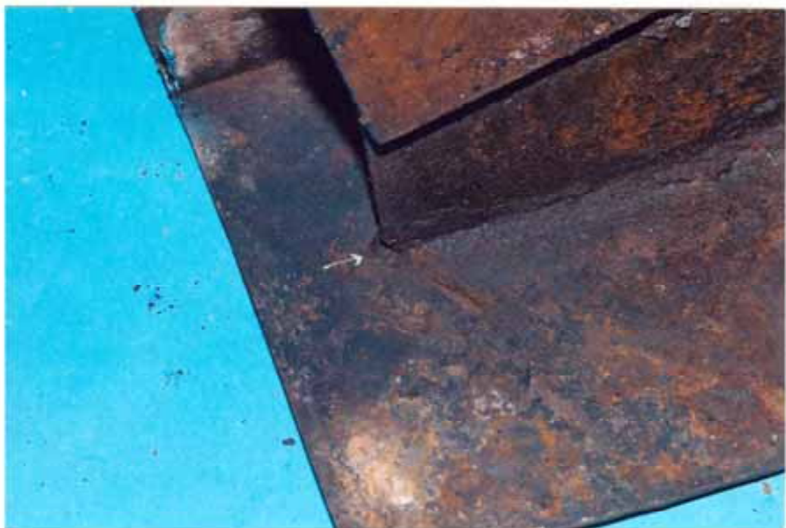
Figure 46: Vee shaped crack (arrowed), which was located at the end of a welded longitudinal attachment.
