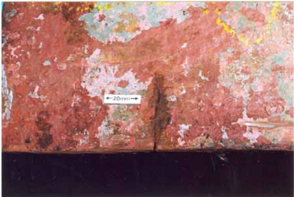
Figure 45: Detail of figure 44 showing second longitudinal crack.
