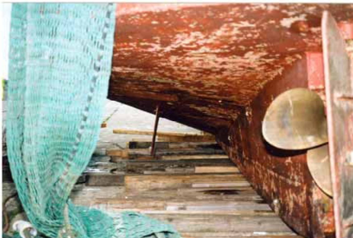
Figure 39: Port side hull and keel, showing largely consumed protective keel mounted anodes and widespread local breakdown of the paint system.
