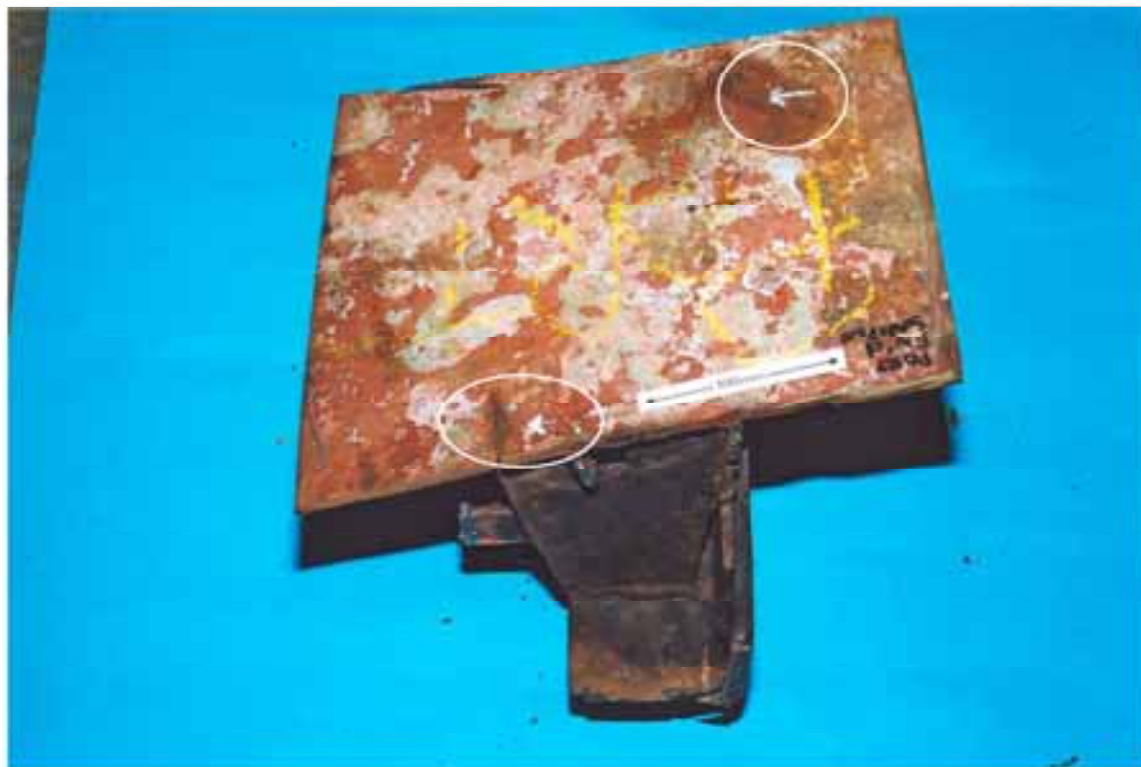
Figure 44: Forward port side sample viewed from the outer sea side and showing the two crack sites arrowed.
