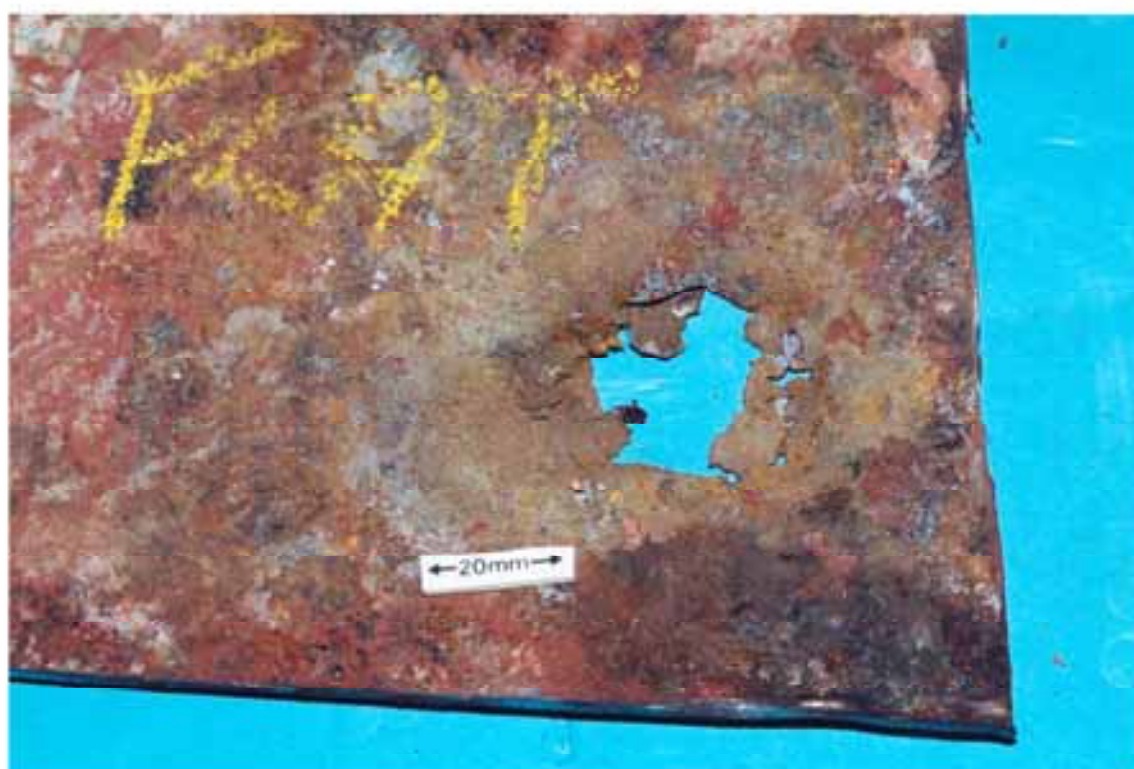
Figure 42: Detail showing perforation site and widespread local breakdown of the protective paint system.
