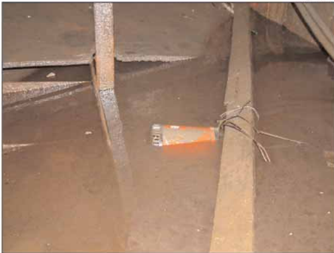
Steering gear compartment submersible bilge pump, lashed to a wooden spar by electrical supply cables
