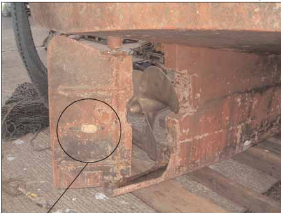
Intact rudder sacrificial anode
