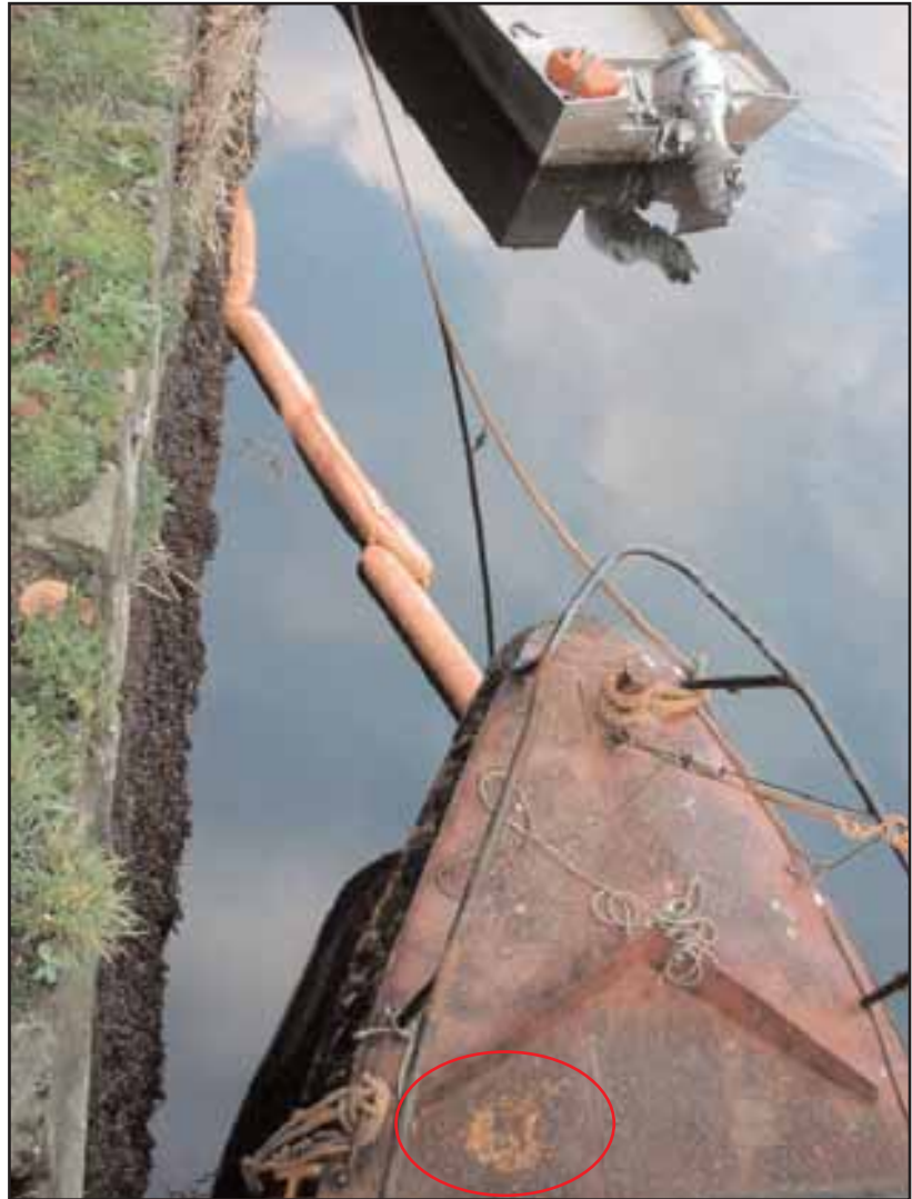
Area of foredeck repair work (circled)
