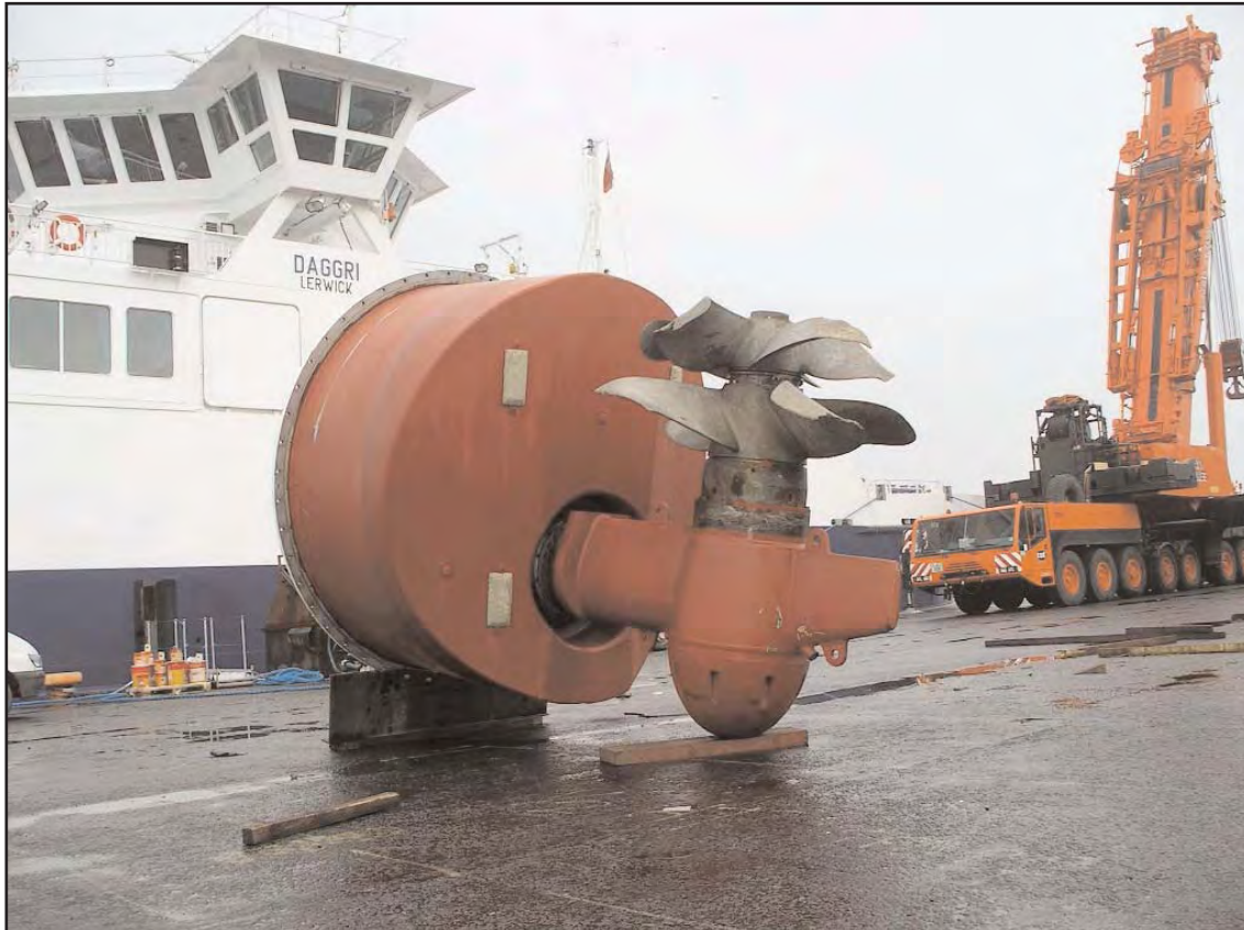
The damaged "forward" thruster unit
