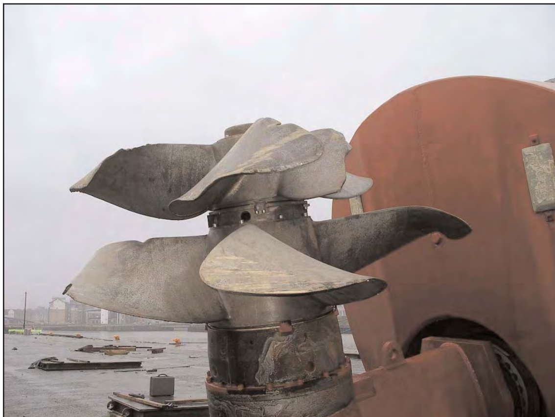
A closer view of the damaged propeller blades
