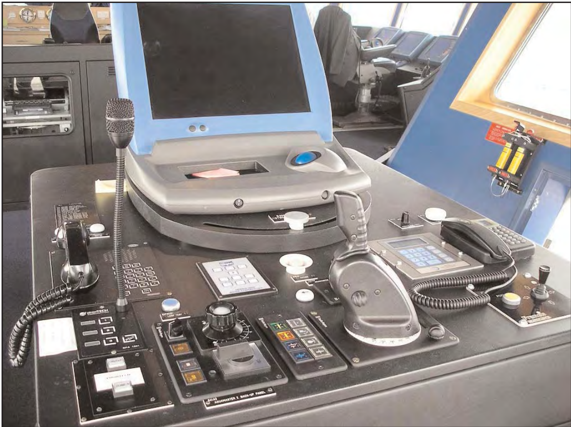
One of the two bridge wing consoles, showing the display and one of the two thruster control handsets
