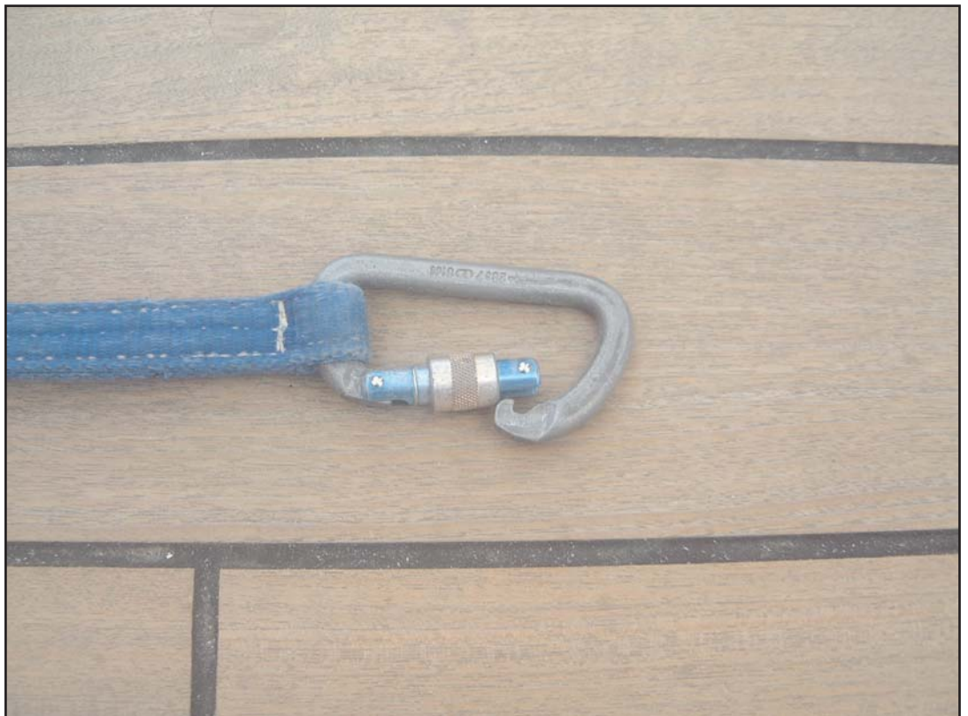
Karibiner clip with screw arrangement partially closed
