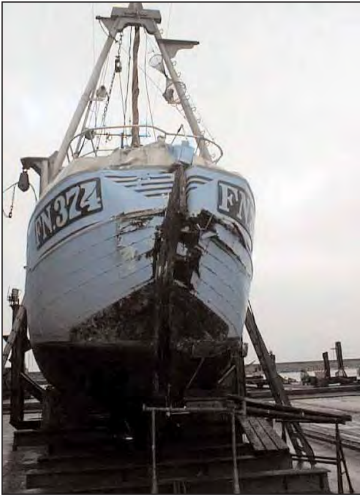
Damage to the bow of Dorthie Dalsøe
