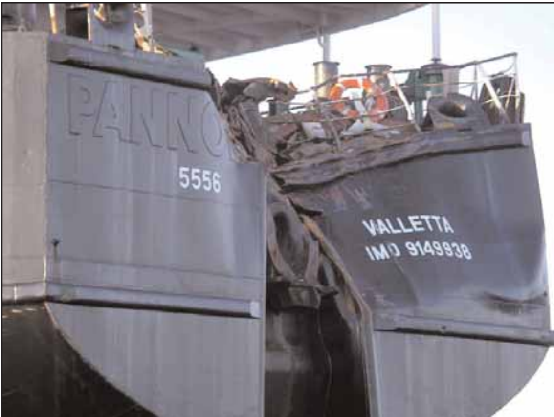
Stern damage to Illeksa
