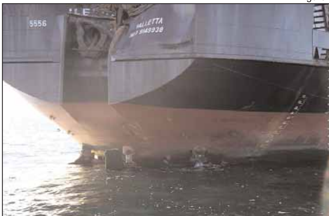
Stern of the Ileksa , showing centre line rudder and, nozzles port and starboard
