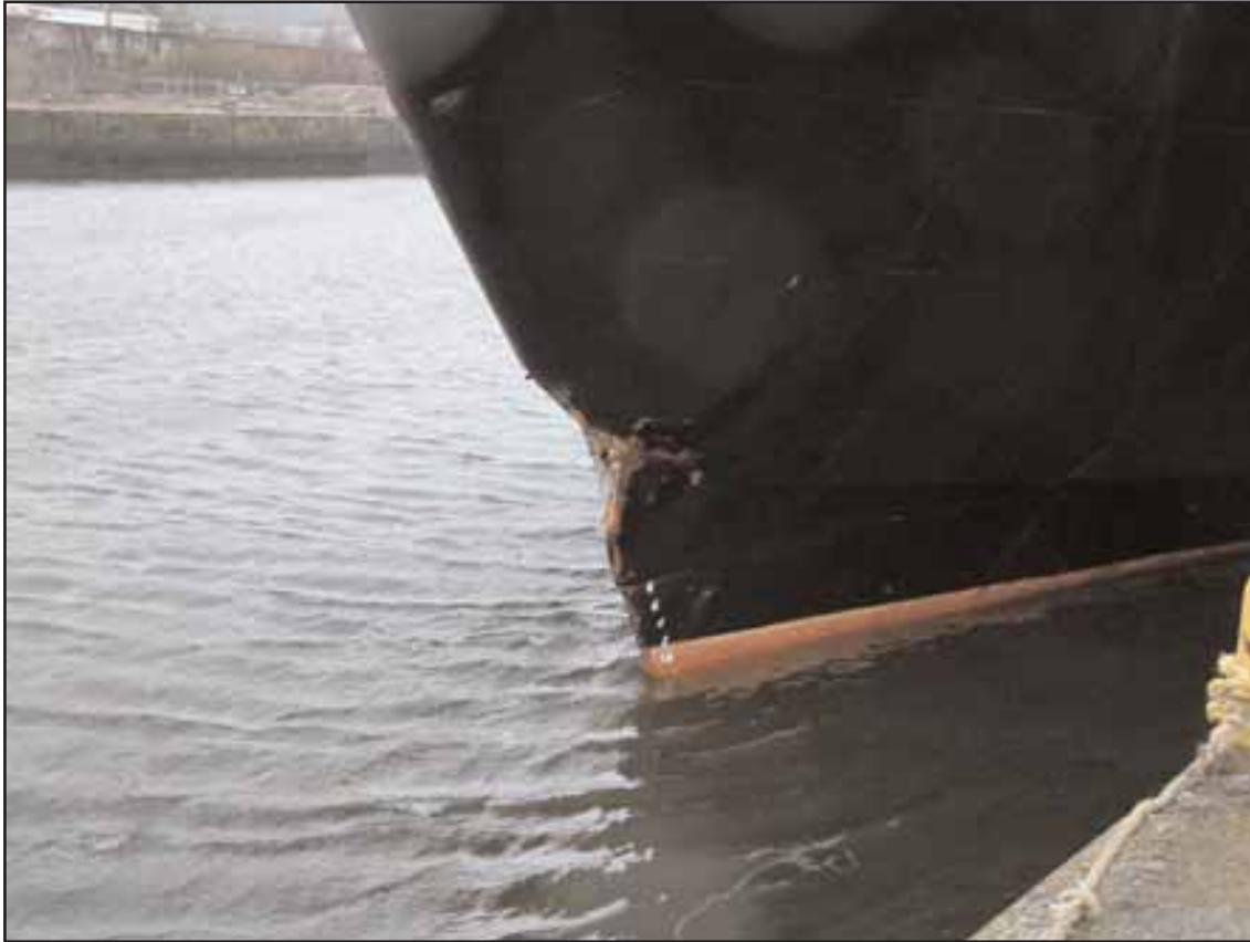
Bow visor damage
