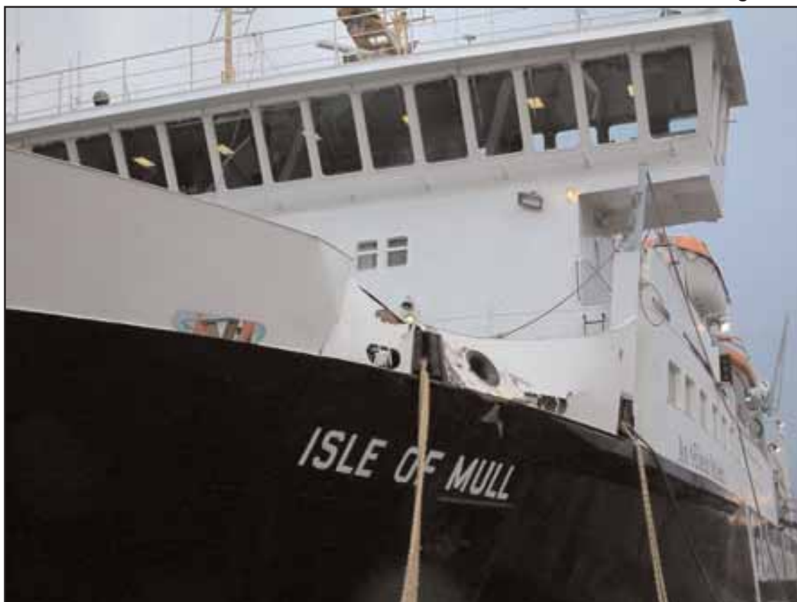
Port focsle damage
