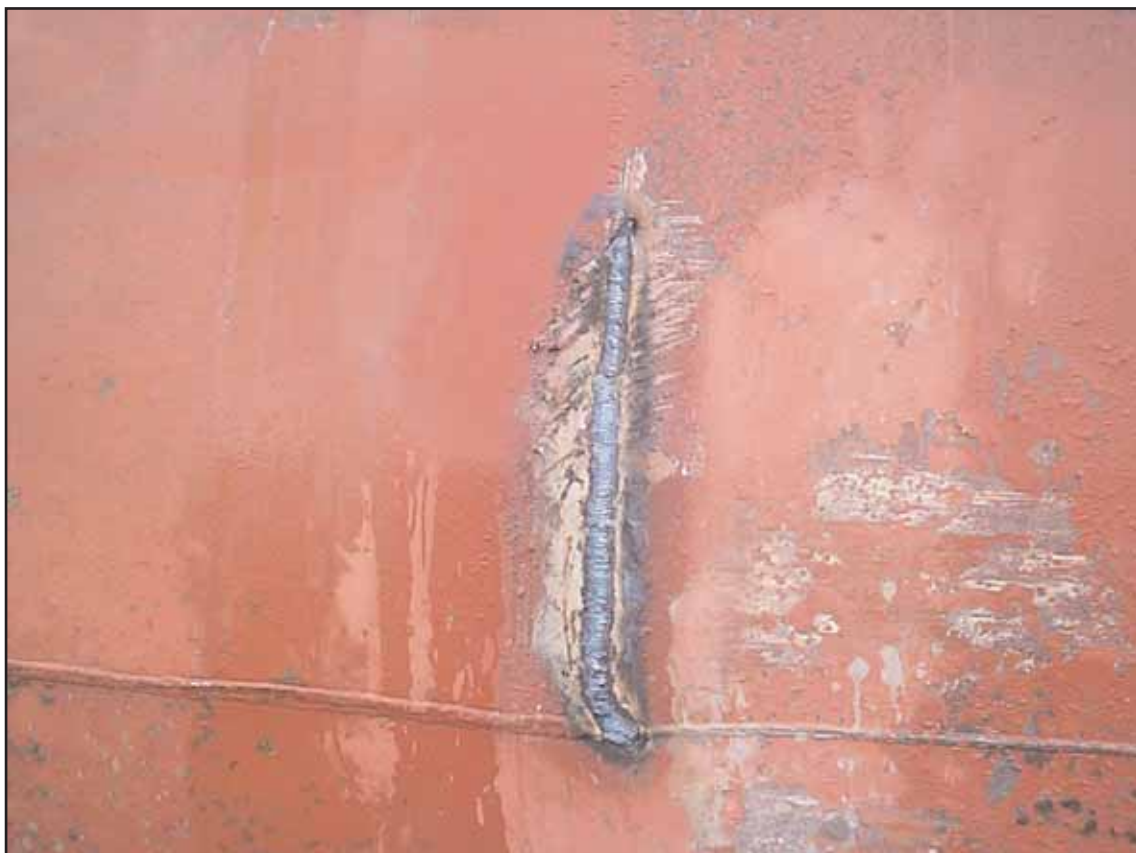
Weld repair to split in the hull
