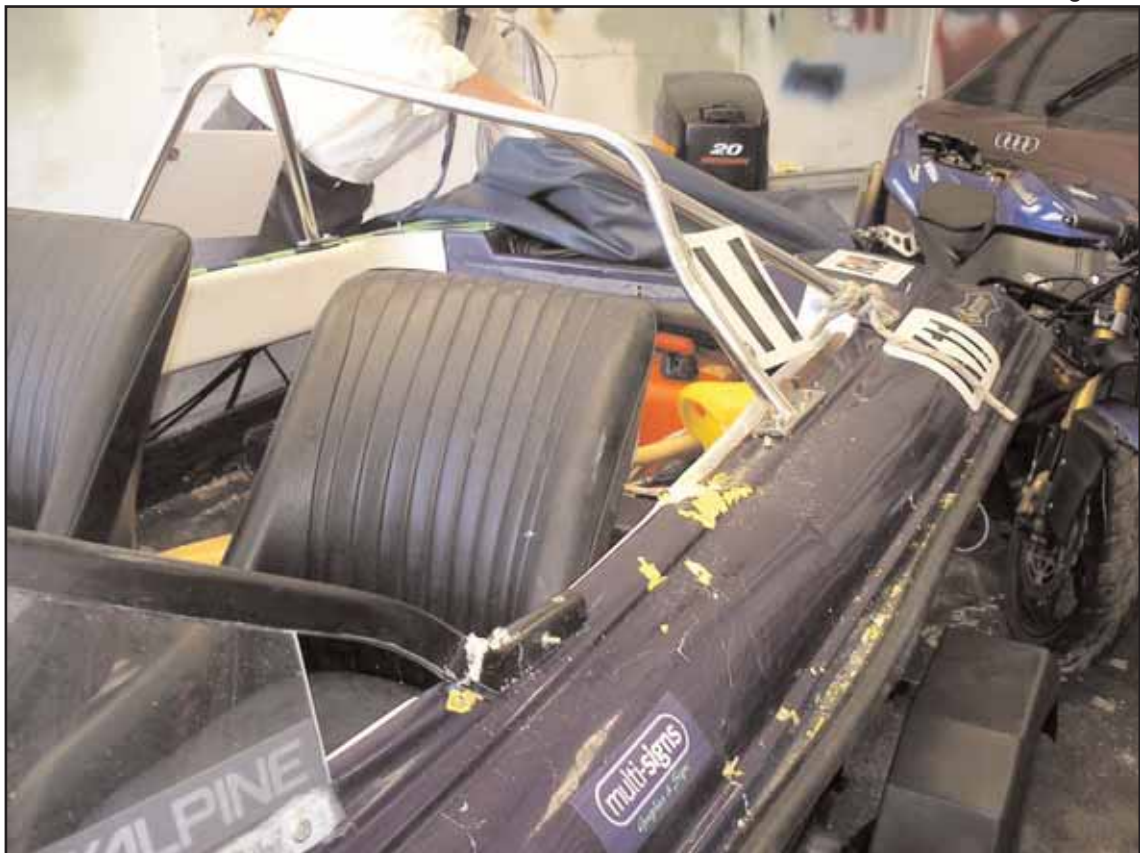
Impact damage to K11
