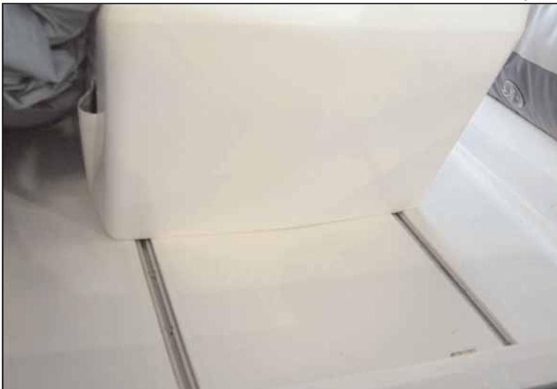
An RY4000 console secured using rail system
