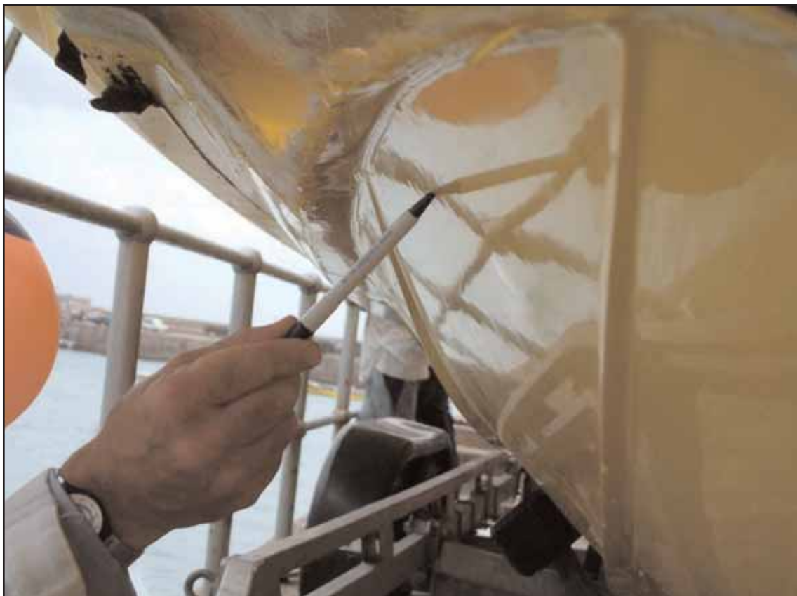
Area of stress cracking
