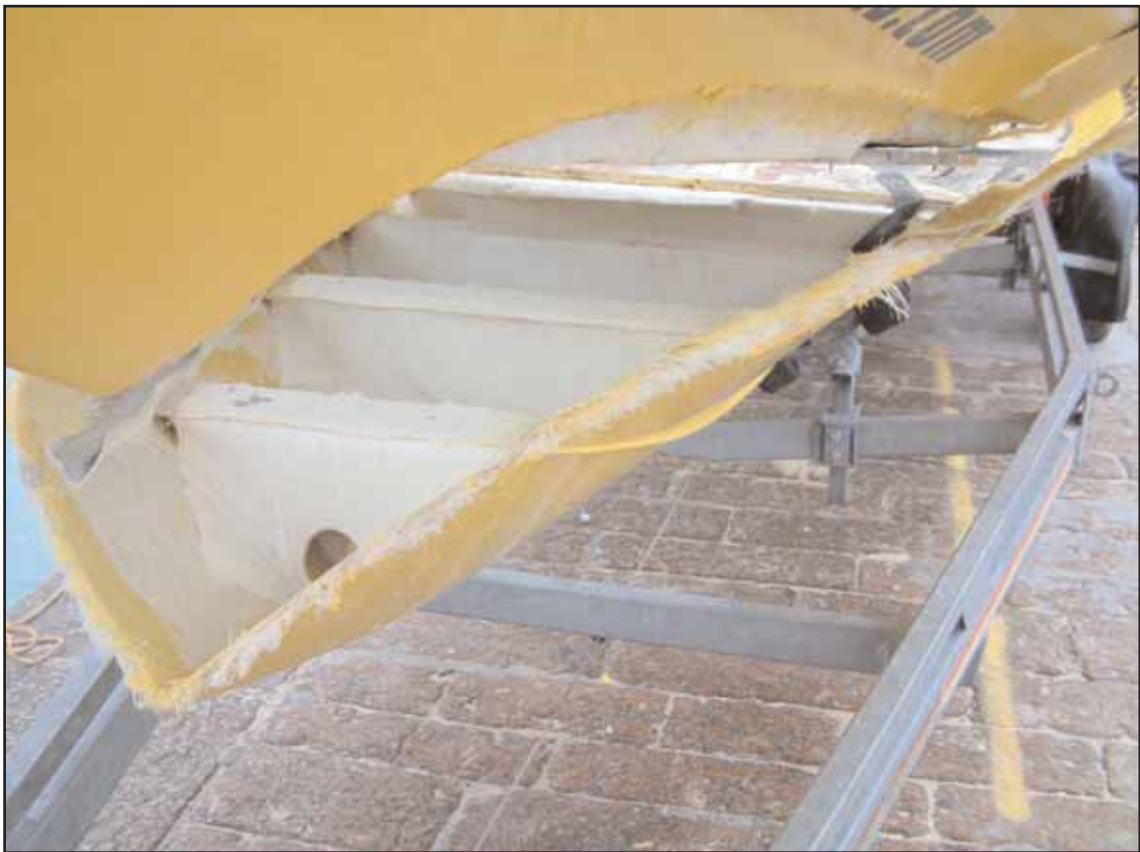
Hull lifted to show extent of damage
