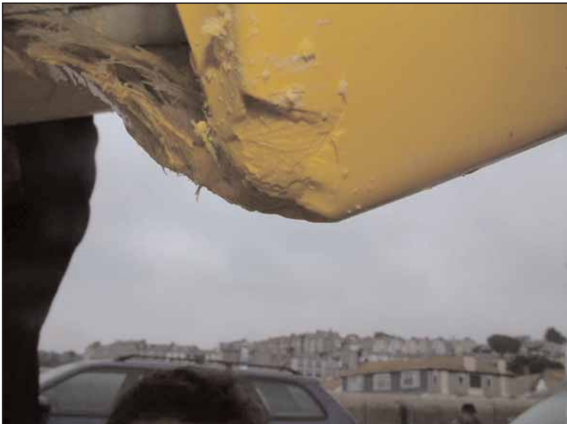
Gel coat detachment at start of reverse chine
