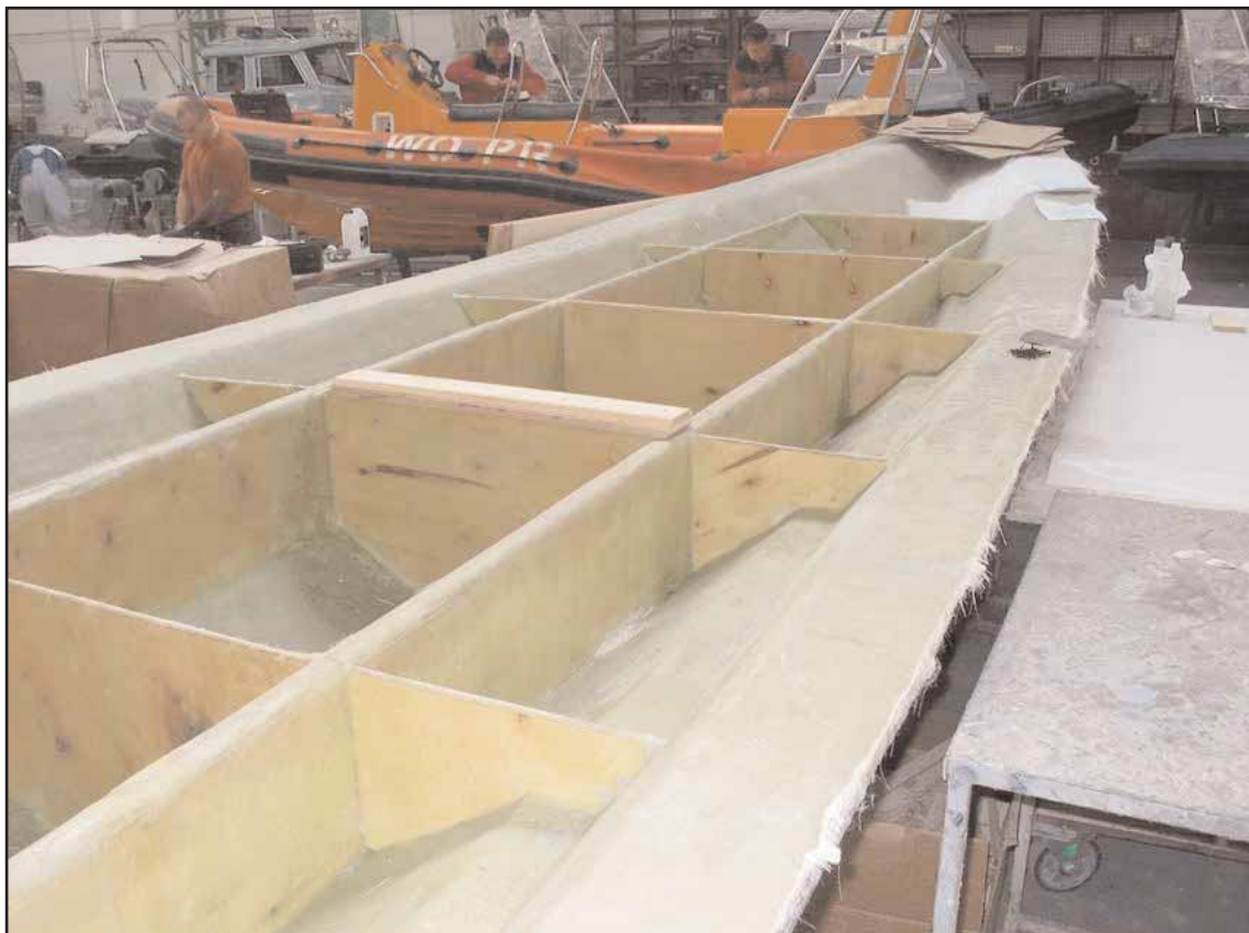
Under deck structural stiffening - Parker RIBs 900RS
