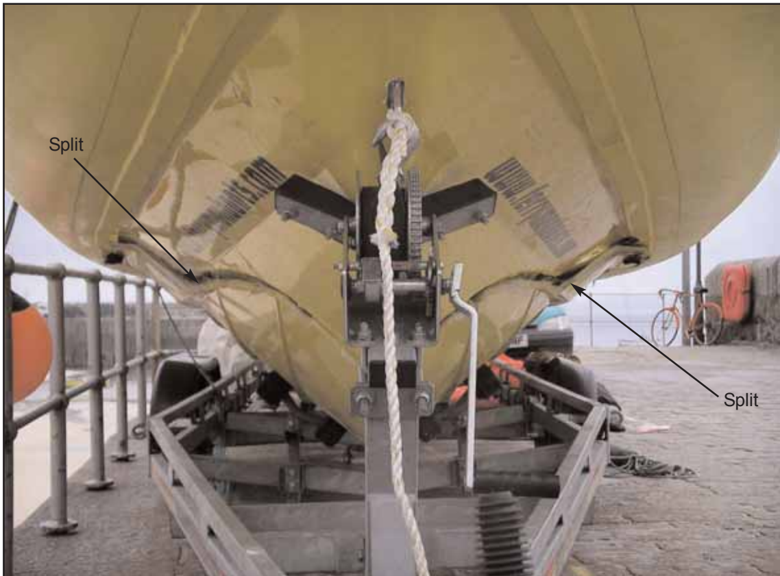
Symmetrical damage from stem
