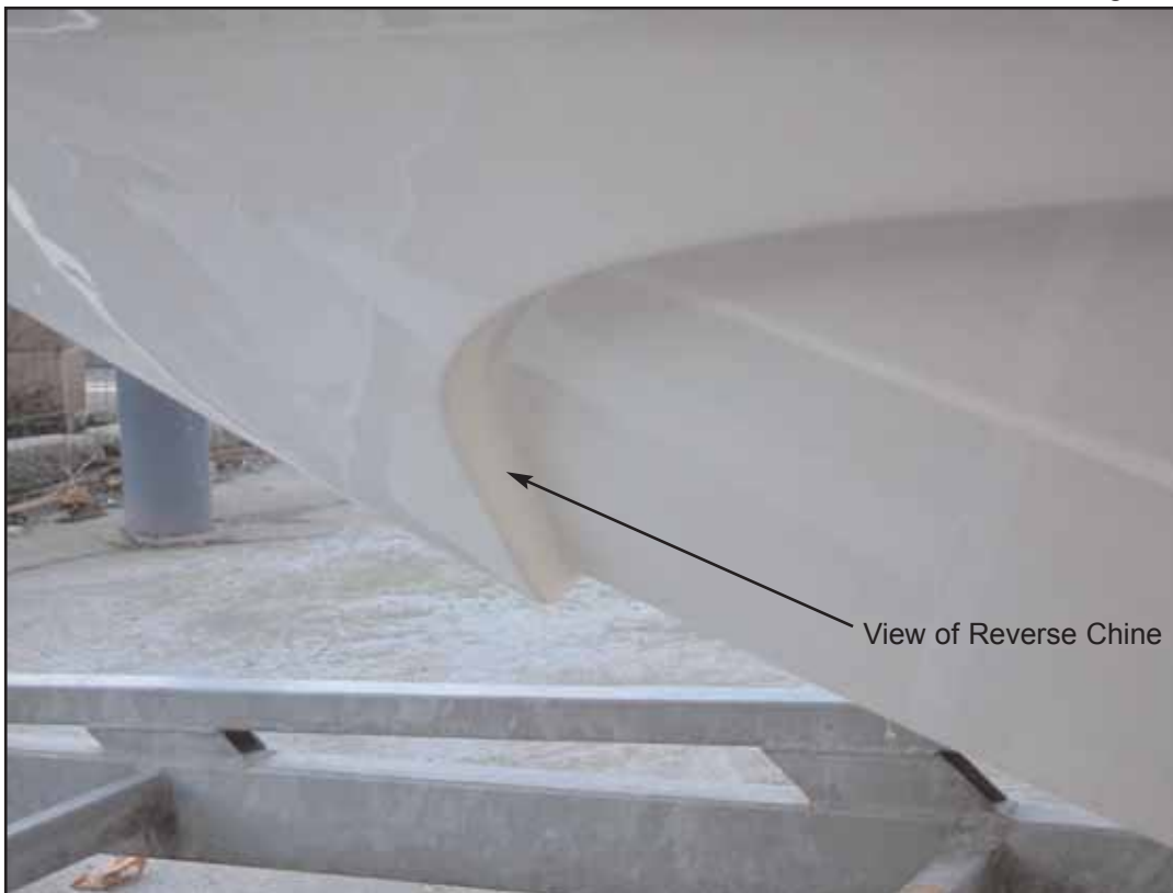
Undamaged reverse chine arrangement
