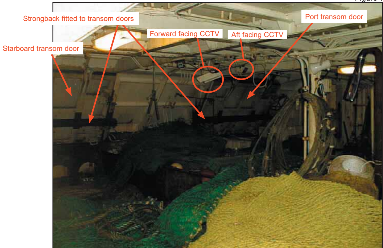
Net drum space on Harvest Hope , looking port aft (February 2003)
