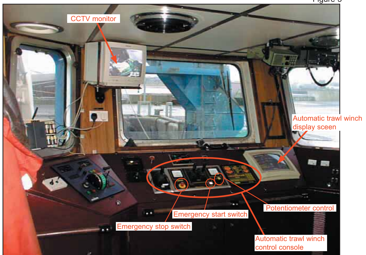
Wheelhouse of Harvest Hope looking aft (February 2003)
