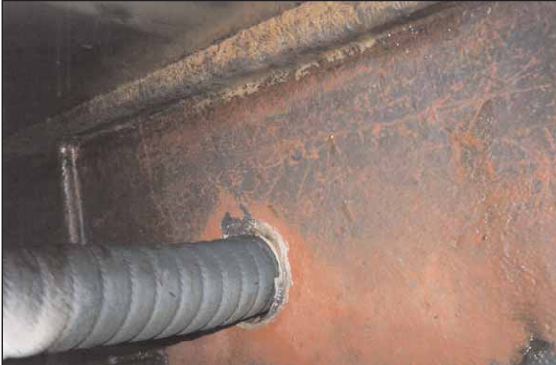
Penetration of aft bulkhead by exhaust hose
