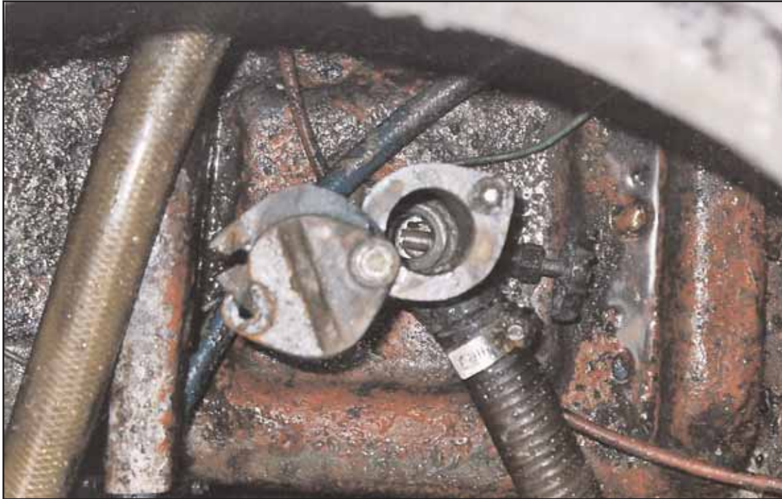
Sea inlet valve, limit of closing
