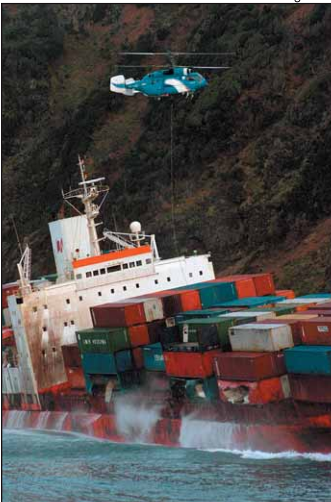
Helicopter operations to remove the hazardous cargo
