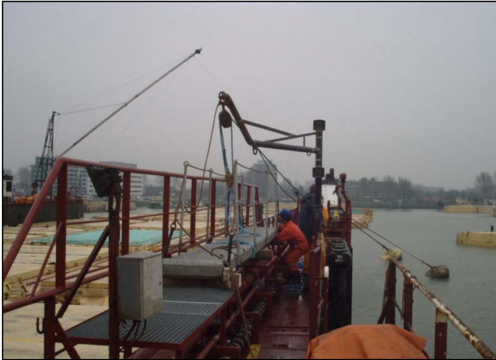
Modified lifting arrangements and extended safety rail
