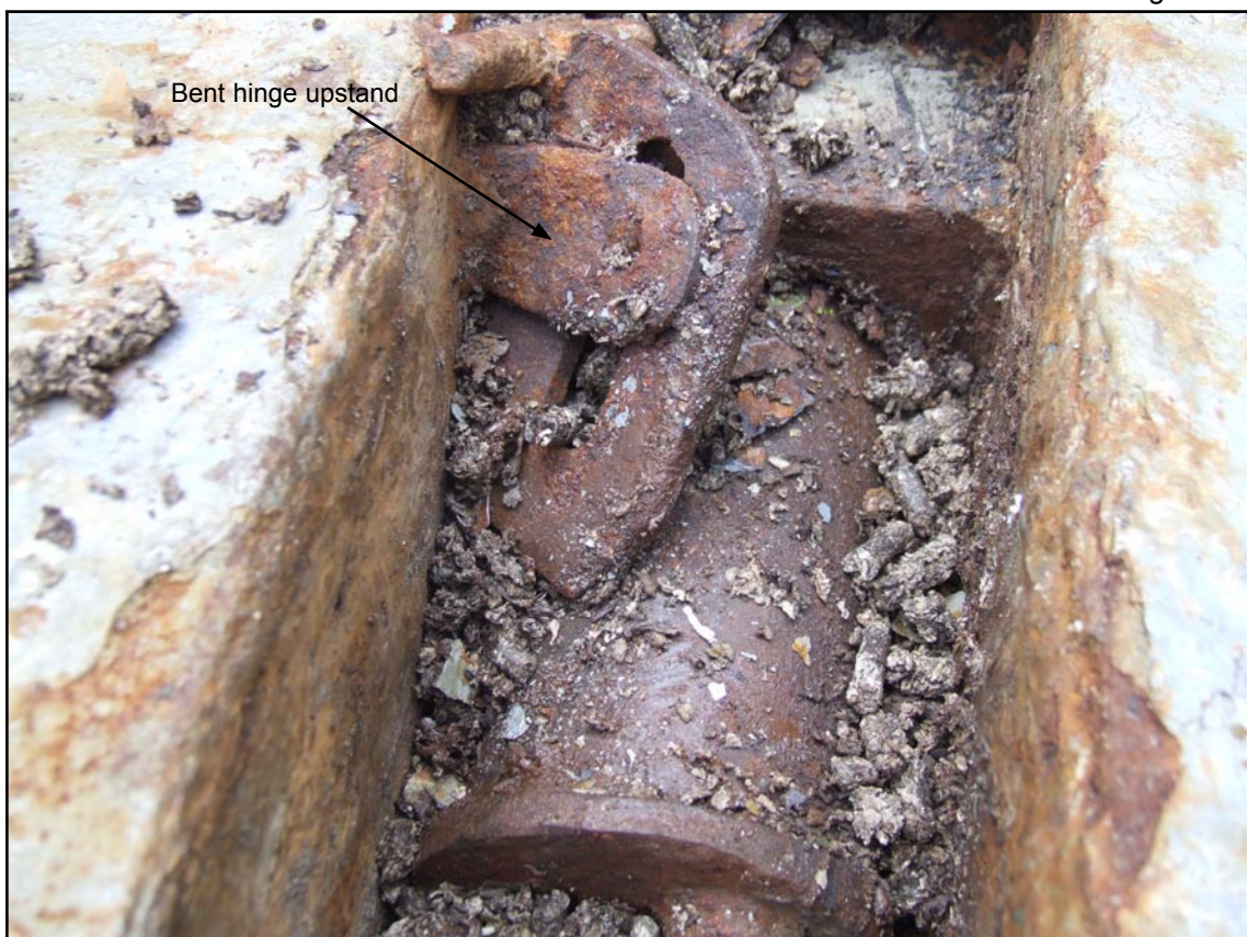
Securing pin starboard upper aft
