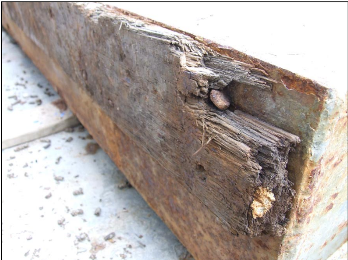
Lower edge of fallen bulkhead
