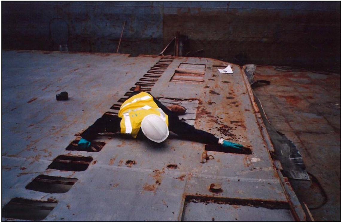
General arrangement of pin operating position, aft bulkhead lying on the bottom of the hold
