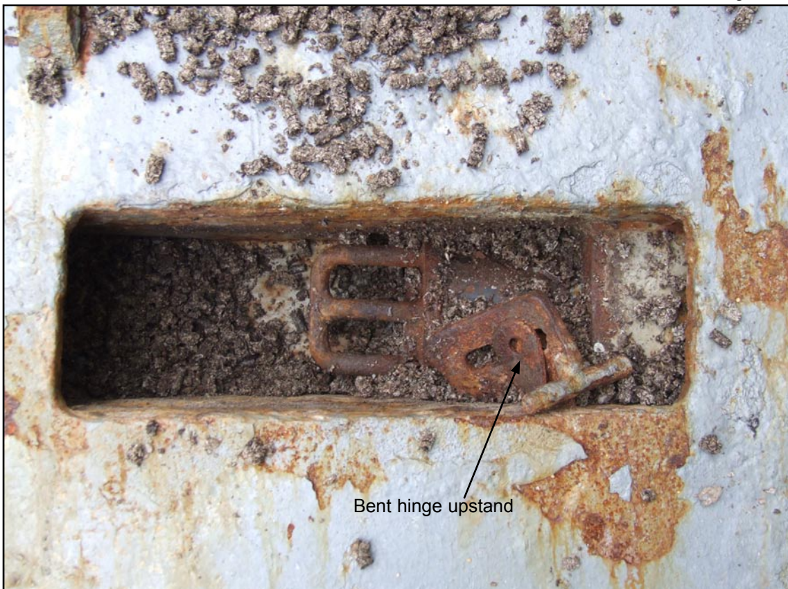
Securing pin port upper aft
