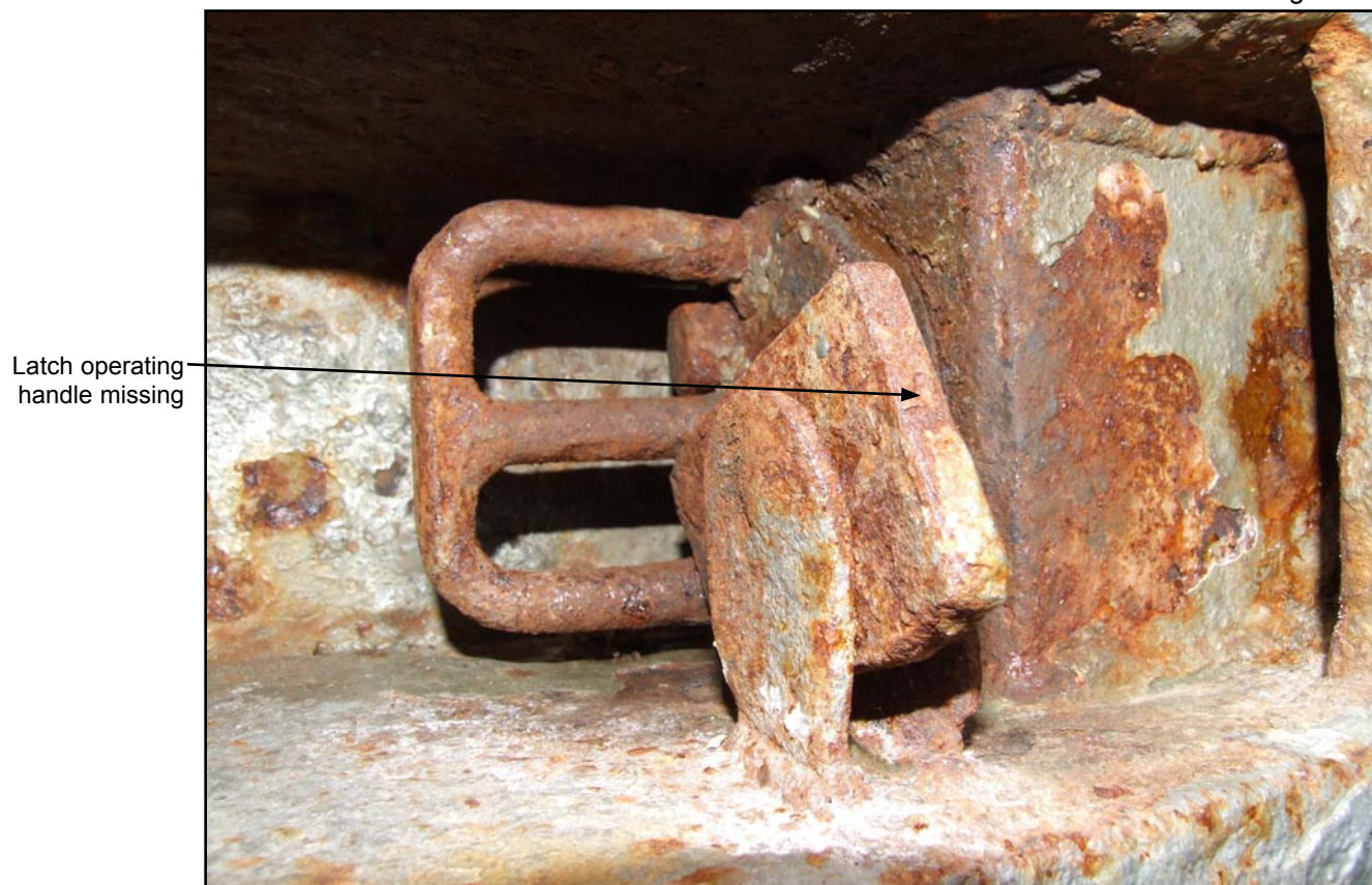
Forward bulkhead, port lower securing pin
